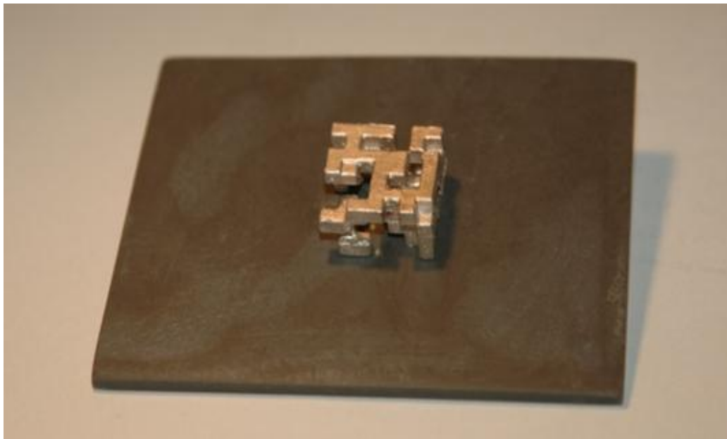
Figure 11: Final built and tested 3D printed antenna metalized with copper paint
