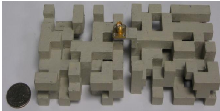
Figure 23: UHF dipole bottom view with silver paint shown next to a US quarter
