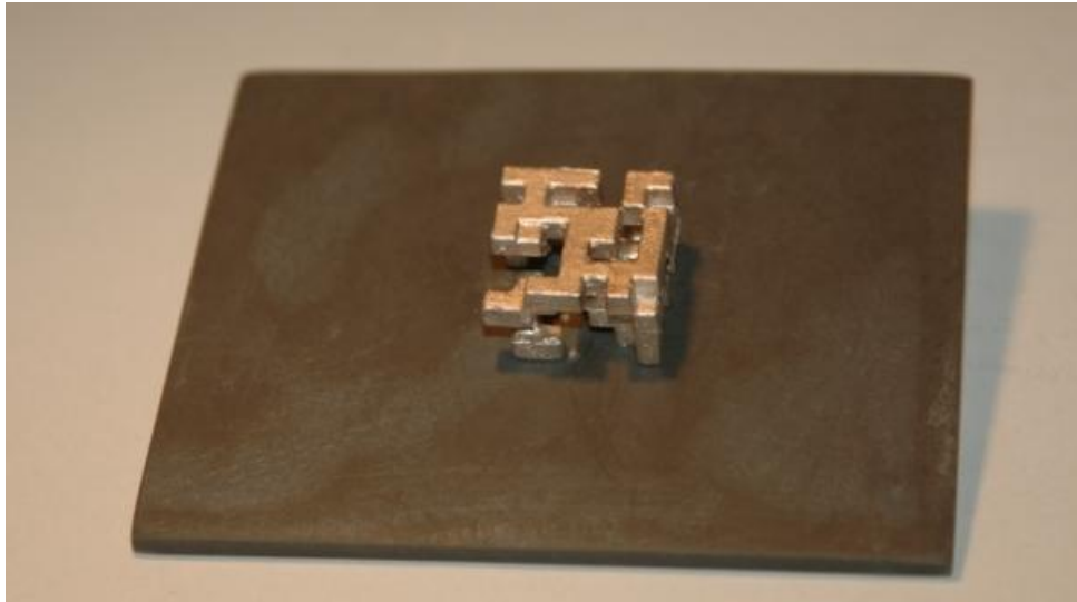
Figure 38: 3D printed cubical antenna above a ground plane, from [14]. © 2012 IEEE. Reprinted with permission.
