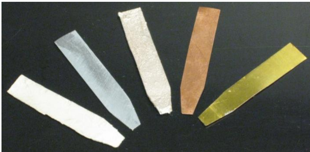
Figure 32: Fabricated antennas from left to right are silver paint, Xyloy®, copper paint, solid copper, and gold plating.
