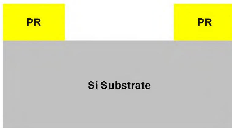
Fig. 4.6: NMOS mesa isolation: mask one lithography
