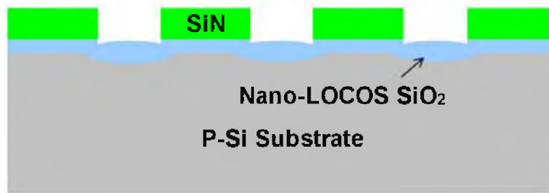
Fig. C.3: The nanostructure first lattices formation: nano-LOCOS
