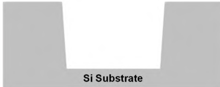
Fig. 4.7: NMOS mesa isolation: silicon trench via RIE
