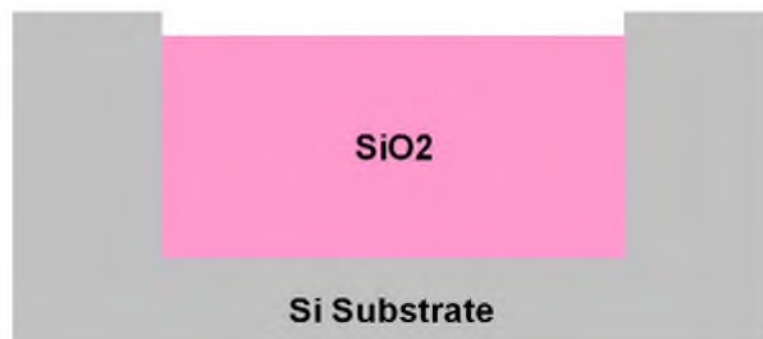
Fig. 4.9: NMOS mesa isolation: CMP
