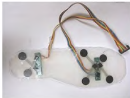
Figure 3.2. Insole sensors in the prototype design.
