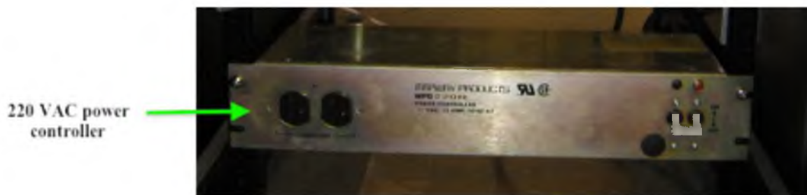
Figure 4.20: 220 V Power Controller. This is a picture of a 220V Mapway power controller module. 220 V power is switched by external power board control lines connected to an internal relay on the control module.
