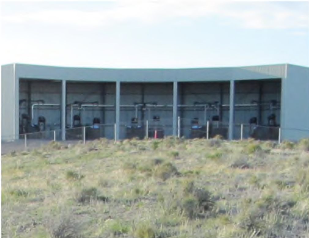
Figure 4.1: TALE Detector Picture. This image shows the five bays of the TALE FD building along with the ten telescopes that compose the detector. Ten mirrors collect light from CR air showers and focus it onto their respective PMT cameras.
