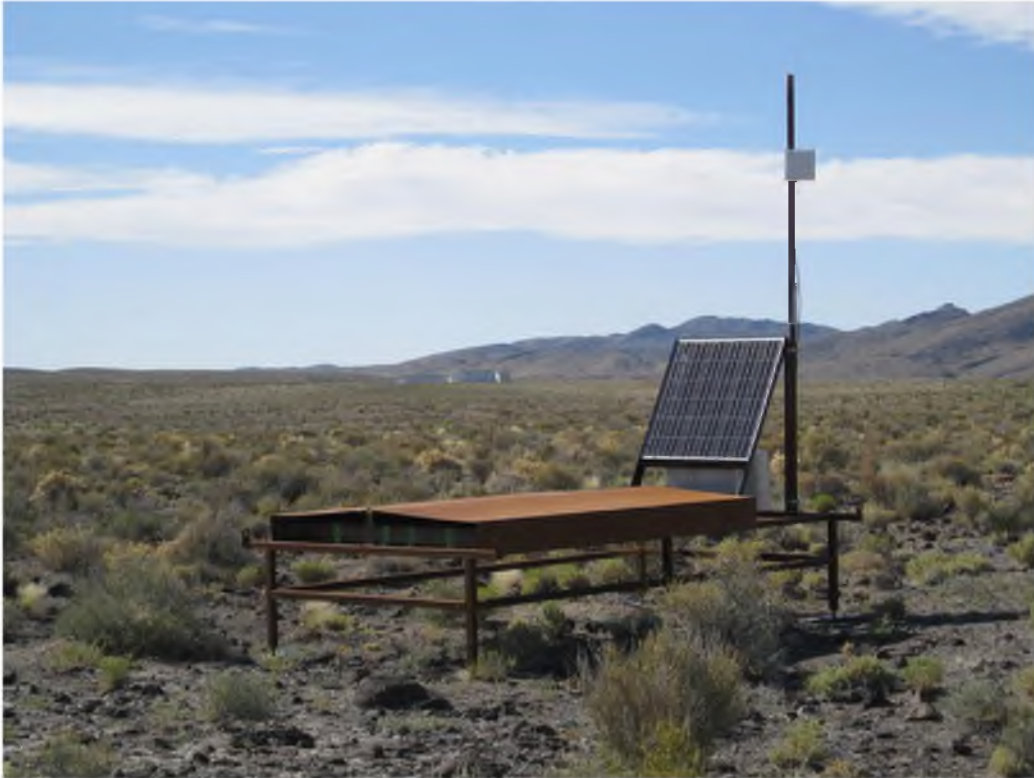
Figure 2.4: Photograph of One of the Telescope Array Surface Detectors. The scintillators are contained in a stainless steel box. The solar panel is used to charge the detectors battery, which supplies power at night. Additionally the communications antenna can be seen on the top of the pole extending from the detector. The scintillating plastic is located on the “bed” of the detector while the control/readout electronics are housed in a box behind the solar panel[11].
