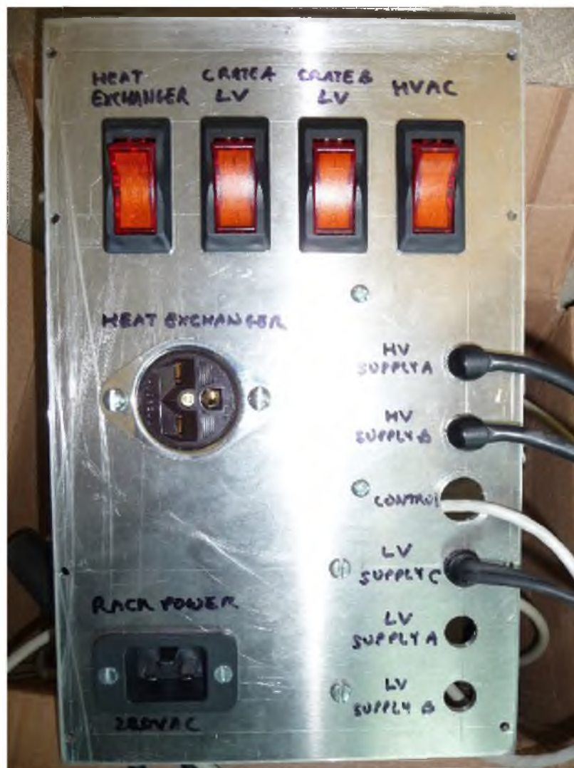
Figure 4.21: TALE Breaker Panel. The HiRes-II panel was composed of GFCI breakers, which frequently tripped when HV power was enabled to the cameras. The new unit (pictured here) is composed of a series of standard over-current breakers and control relays. The internal relays in the breaker panel allow the power control board to determine when HV and LV supplies are provided power.
