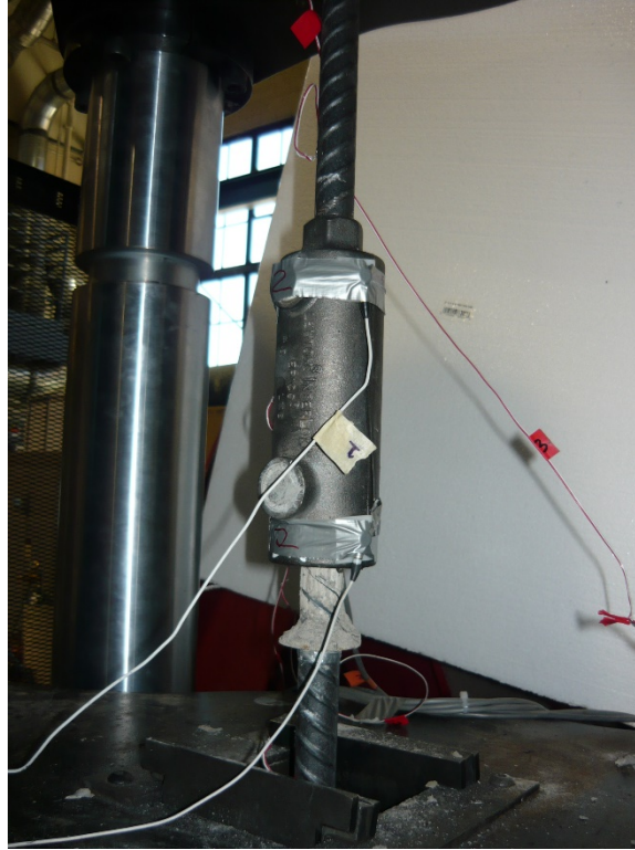
Failure of air test specimen in testing apparatus
