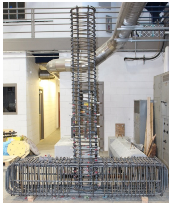
Specimen CIP reinforcing bar cages
