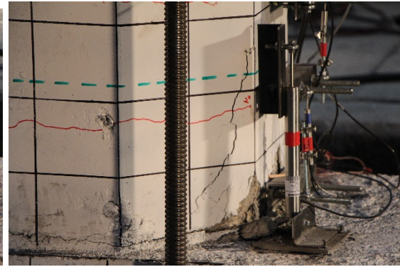
Damage state at 3% drift ratio
