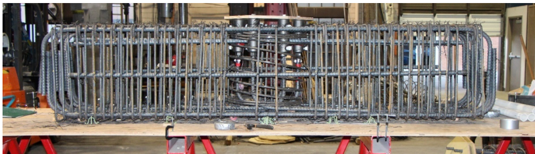
Specimen FGSS-2 reinforcing bar cages
