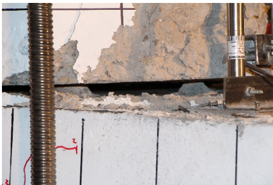
Bar pullout during 6% drift ratio
