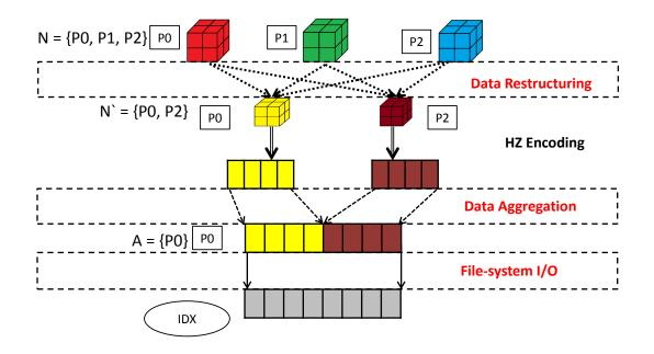
Figure 7.1: Block diagram showing the three I/O phases of PIDX – restructuring, aggregation, and file I/O.
