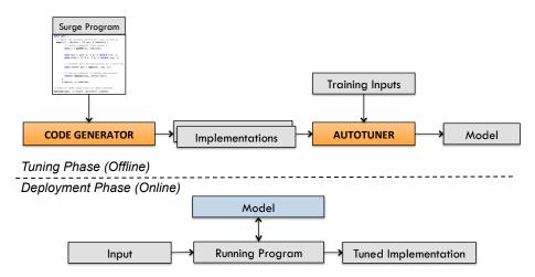
Figure 5.4: Overview of the Surge framework and its interaction with Nitro.
