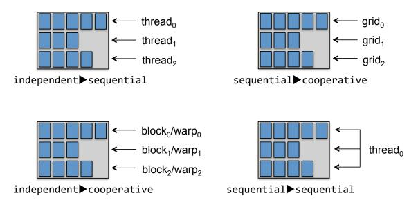
Figure 5.3: How various SpMV schedules may be implemented in CUDA. In this example, the input matrix (gray boxes) has 12 nonzeros (blue boxes) and 3 rows.
