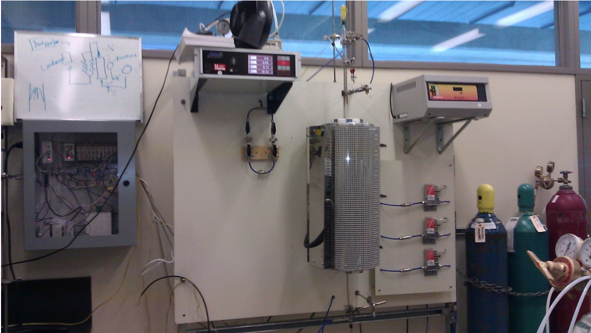
Figure 9: Chemical-looping fluidized-bed reactor system at the University of Utah.
