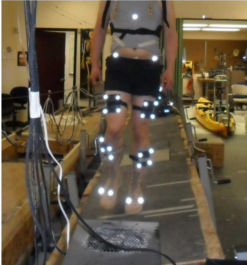
Figure 3-2 Participant walking back on tilted track (wearing markers) program to identify the body landmarks necessary to establish the body segments and determine the entire CoM for the person.
