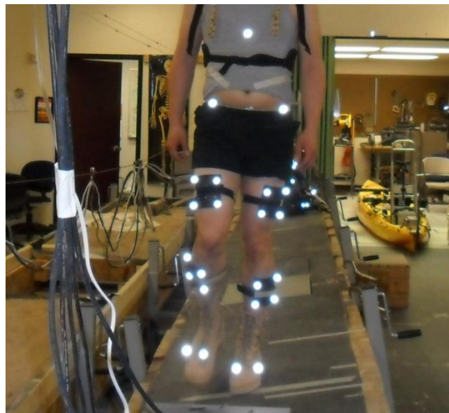
Figure 2-2 Participant walking back on tilted track (markers identify body and foot location so equipment can calculate center of mass and center of pressure). Note the rectangular force plates in the middle of the track behind the participant.
