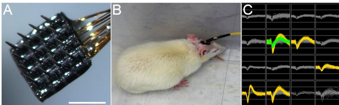
Fig. 2.1. (A) UEA before implantation. Scale bar = 1 mm. (B) Electrophysiological recording session with an awake and behaving rat implanted with a UEA. (C) Representative waveforms from a recording session in which single unit action potentials were isolated on 5 of the 16 microelectrodes.
