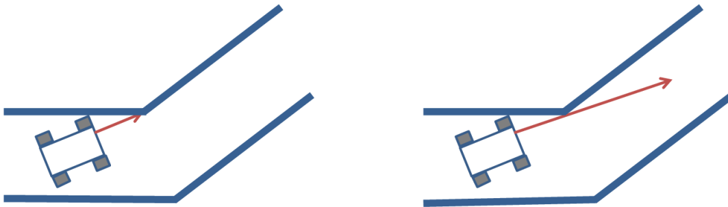
Figure 2.10: IR sensor reading fluctuation in the corner scenario.
