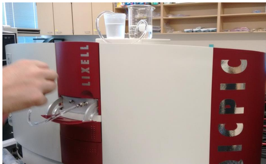
Figure 3.8: Sample delivery system using siphon system.
