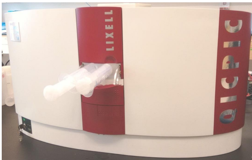
Figure 3.6: Sample delivery using two leur lock syringes in parallel.
