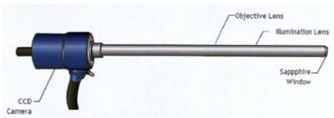
Figure 3.1: Particle Vision & Measurement probe (source: Mettler Toledo PVM manual).
