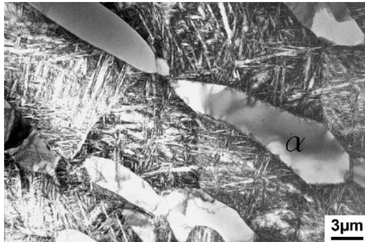
Figure 2.12: TEM micrograph of Ti-6Al-4V recrystallized at 950 °C to form a bi-modal microstructure (reproduced with permission of Springer via RightsLink/Copyright Clearance Center) 34 .
