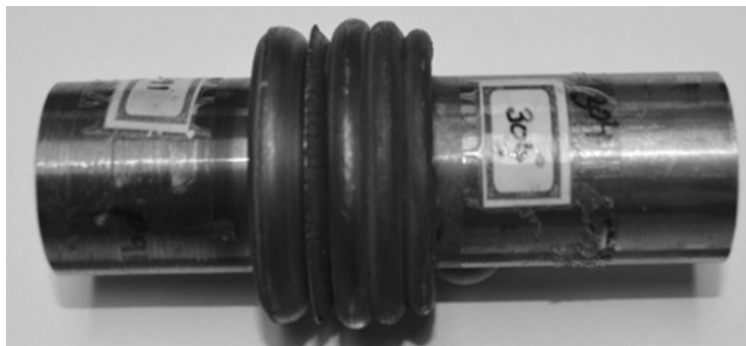
Figure 3.21 P91/AISI 304 weld transition joint produced using friction welding employing multiple interlayers.
