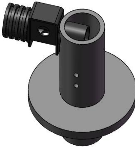
Figure 2.2 The standard sensor with no modifications inserted into the flow sensor housing
