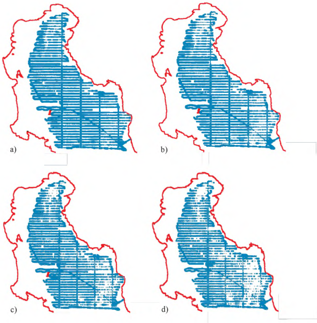
Figure 22. Calculated rugosity values for 50, 100, 250, and 500-sample intervals, north part of Great Salt Lake, Utah. Larger diameter circles indicate larger calculated rugosity. Rugosity based on a) 50-sample interval, b) 100-sample interval, c) 250-sample interval, and d) 500-sample interval.
