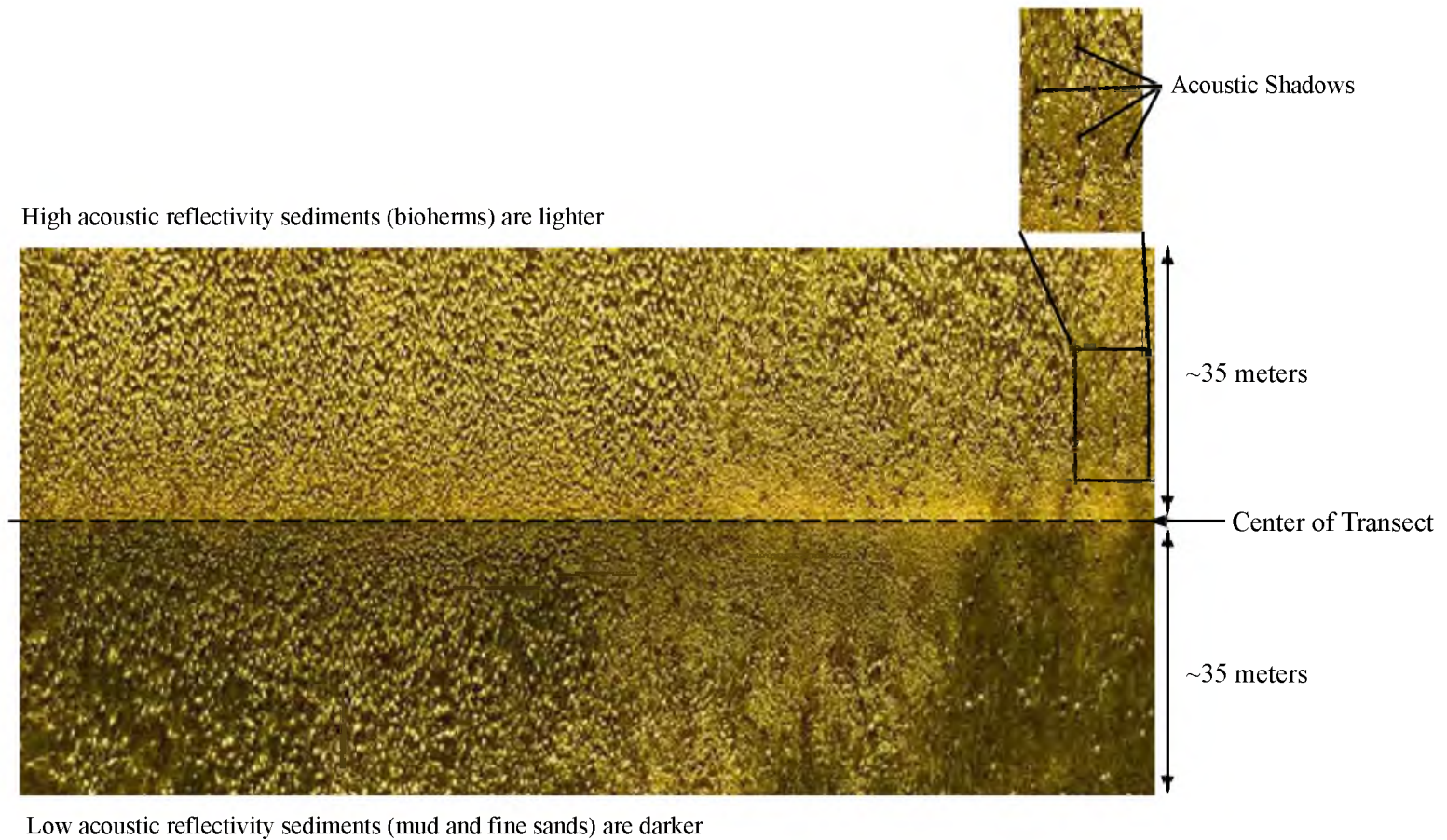
Figure 19. Side scan sonar image showing microbial bioherms (lighter, high acoustic reflectivity) occurring with fine-grained sediments (darker, low acoustic reflectivity) in Great Salt Lake, Utah. Distortion due to the varying high salinity is apparent in the image as are high intensity returns along nadir where the two sides on the sonar imagery are joined.
