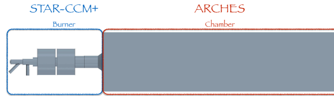
Figure 2.8. L1500 simulation coupling between Arches and STAR-CCM+
