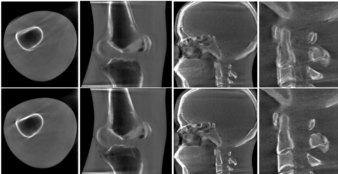
Figure 2.9. Knee (left two columns) and skull (right two columns) physical phantoms reconstruction results. The top row consists of OSEM reconstruction without any geometry estimation. Both reconstructions exhibit ghosting artifacts where a structure appears twice in the reconstruction due to miscalibration. In particular, double edges exist on the front of the femur and back of the tibia in the knee phantom and around the skull boundary and the vertebrae on the skull phantom. The bottom row shows the OSEM reconstruction with geometry estimation. In these reconstructions, the ghosting artifacts are eliminated.
