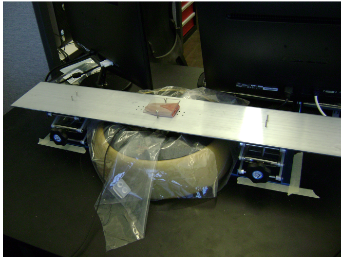
Figure 2.4. Experimental setup. The experimental setup consists of the MLHD, custom tactor (not seen), jack stands, and aluminum platform. The tongue sample is secured to the center of the aluminum platform. A slot in the center of the platform allows the tactor to make contact with the tongue sample. The jack stands are fitted with two screws which fit through corresponding holes in the platform. The screws secure the platform to the jack stands and masking tape was used to mark proper placement of the jack stands.
