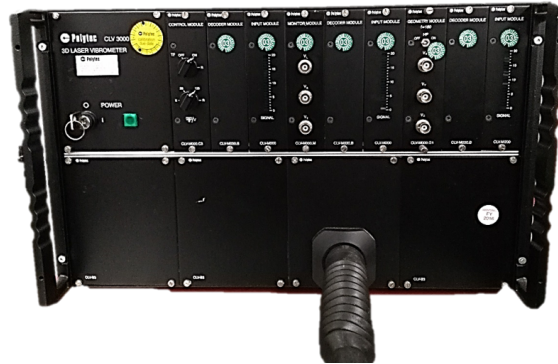
Figure 2.6. Polytec laser vibrometer controller.
