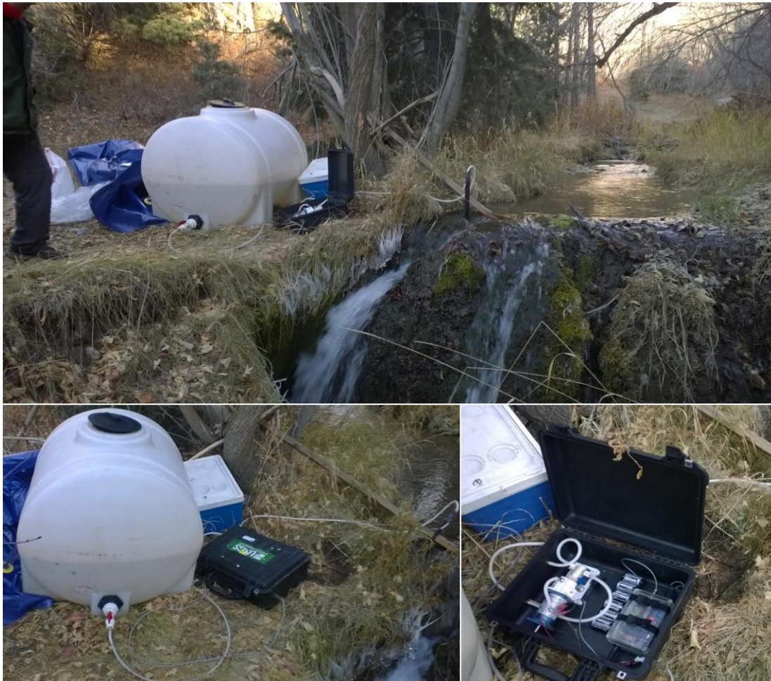
Figure 7. Photos of the set up for the bromide injection test. The top photo shows the overall setup at the top of a small cascade. The bromide solution is injected into the top of the cascade which allows for rapid mixing with the stream. The lower left picture shows the tank and pump setup. The lower right shows a close up of the pump used. The pump was programmed to inject 100 mL/min. (Photos by Stewart Gubler)
