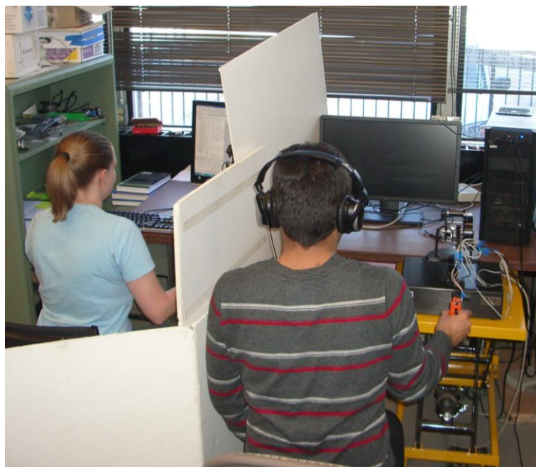
Figure 4.18. Experimental setup for the teleguidance procedure. The participant (on the right side) cannot see or hear the operator or see the motion cues provided to the operator on the computer screen. The expert operator cannot see the participant, but can hear if they need to redo a specific trail within the series of motions.
