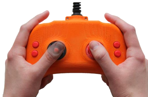
Figure 2.3. A custom-made game controller with skin stretch feedback provided on the front of the device, underneath the thumbs.
