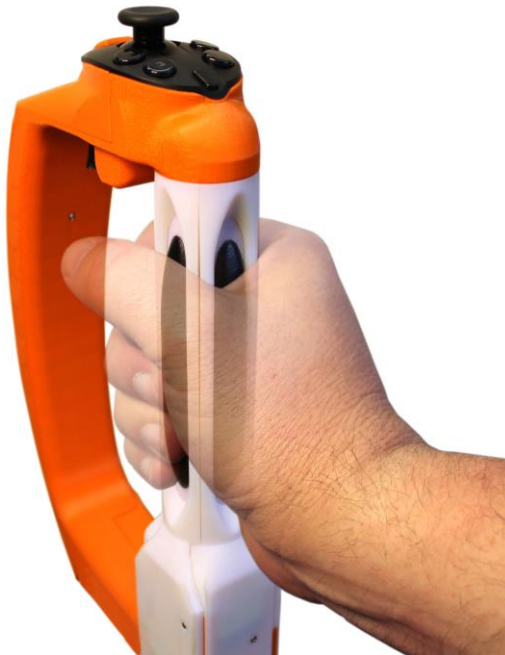
Figure 3.2. The power grip skin stretch feedback device. A user grips the handle, and the tactors (shown in black) slide against the palm and fingers.
