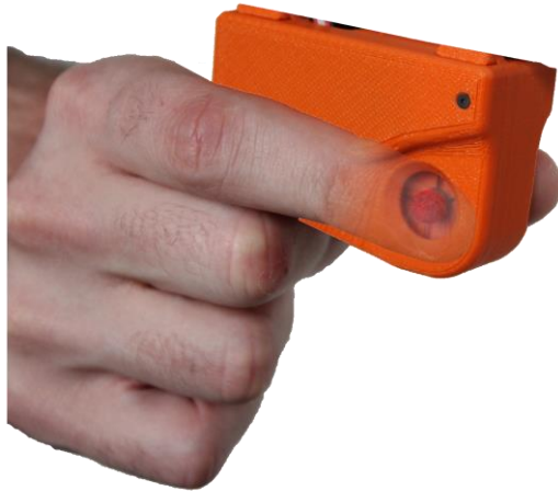
Figure 3.1. The precision grip skin stretch factor device. A user places their thumb over one factor, and their index finger over the second factor (shown in red).
