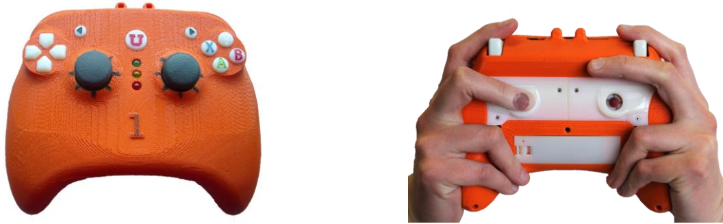
Figure 2.4. A custom-made game controller with skin stretch feedback provided on the back of the device, where the middle fingers rest.
