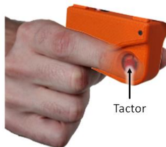
Figure 3.4. An external view of the precision grip skin stretch feedback device. The user holds the device in their hand, making contact with each tactor with his/her index finger and thumb.
