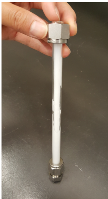
Figure 3.7 Photo of the grown monoliths synthesized in a polycarbonate tube.
