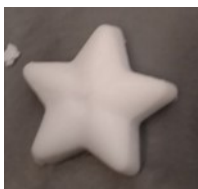
Figure 3.6 Photos of the monoliths synthesized in a silicone ice cube.
