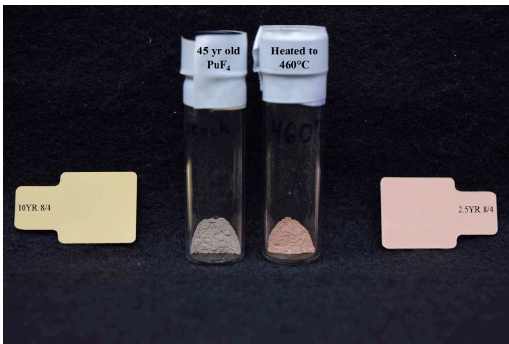
Figure 3.4 Comparison of \text{PuF}_4 that has undergone near 50 years of radiolysis (left) with that of 460^\circ\text{C} annealed \text{PuF}_4 (right); Munsell color chart tabs are placed next to the samples for further comparison (10YR 8/4 right tab and 2.5YR 8/4 left tab).
