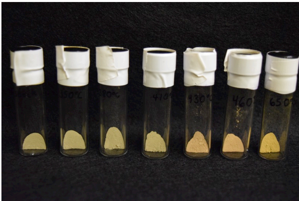
Figure 3.3 0.5g samples of \text{PuF}_4 annealed at (from left to right) 350°C, 380°C, 410°C, 430°C, 460°C, 620°C, and 650°C. There is a clear transition in the material from grey at a predominately amorphous state, to pink at a predominately crystalline state (from left to right). A third color change, orange, is illustrated in the 650°C (far right) sample.
