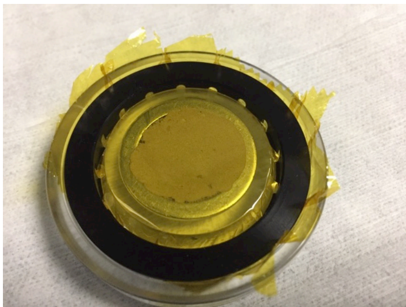
Figure 3.6 1.0g sample of 460°C annealed \text{PuF}_4 within a Bruker A100B33 X-ray diffraction specimen holder sealed with 3511 Kapton®. A 0.755-inch inner diameter 1100 series aluminum washer was fit into the A100B33 well. This reduced the well's volume by near 25 percent. This sample exhibited a more suitable surface flatness for X-ray diffraction analysis.
