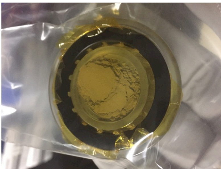
Figure 3.5 1.0g sample of 350^\circ\text{C} annealed \text{PuF}_4 within a Bruker A100B33 X-ray diffraction specimen holder sealed with 3511 Kapton®. Clearly, 1.0g of \text{PuF}_4 was not adequate to fill the entire specimen well. Therefore, for all subsequent specimens, 0.755-inch inner diameter 1100 series aluminum washers were fit into each A100B33 well. This reduced the well's volume by near 25 percent.
