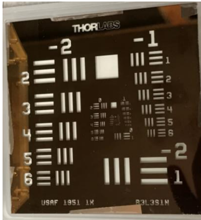
Figure 5.7 Photograph of 1951 USAF test resolution chart (R3L3S1N) from Thorlabs [27].
