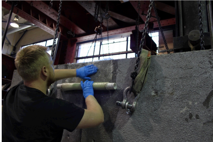
Figure 4.13 – Connection step 2: Lay-up wet GFRP laminas.
