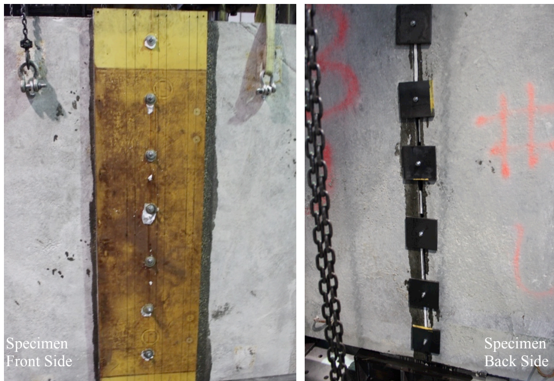
Figure 4.2 – Method of applying pressure during curing to GFRP composite connection.
