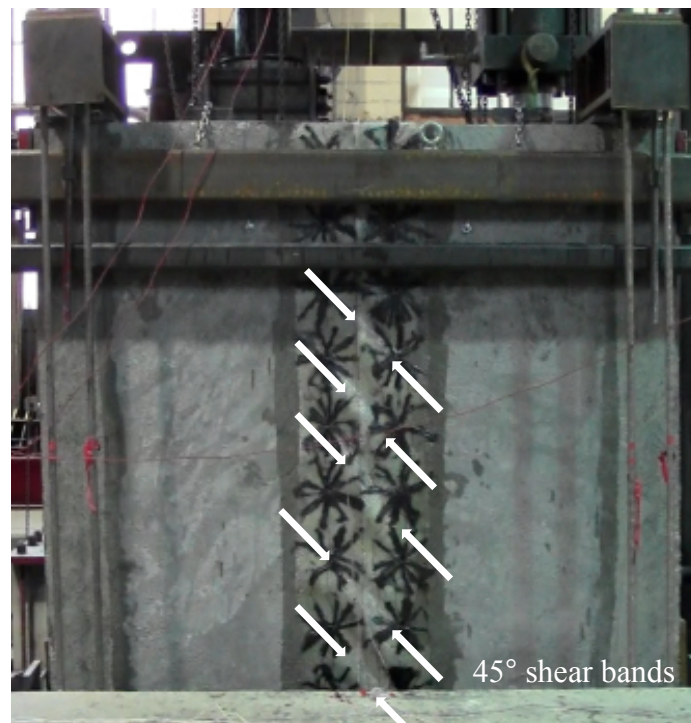
Figure 4.30 – Test #4 connection during failure.
