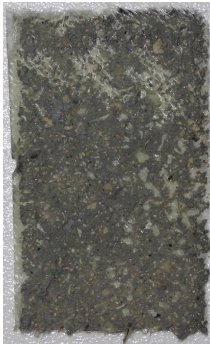
Figure 3.27 – Typical delaminated GFRP concrete removal for multiple-pass washed specimen.
