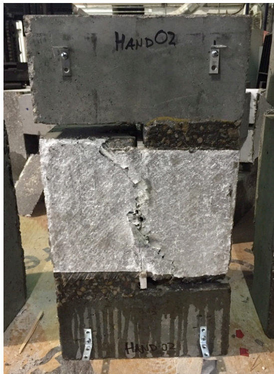
Figure 3.18 – Typical failure with scabble method specimens.
