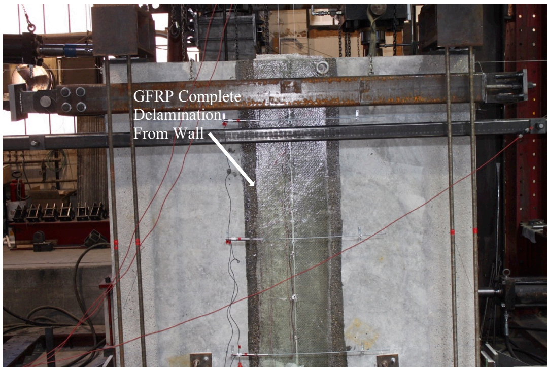
Figure 4.36 – Test #6 connection failure.
