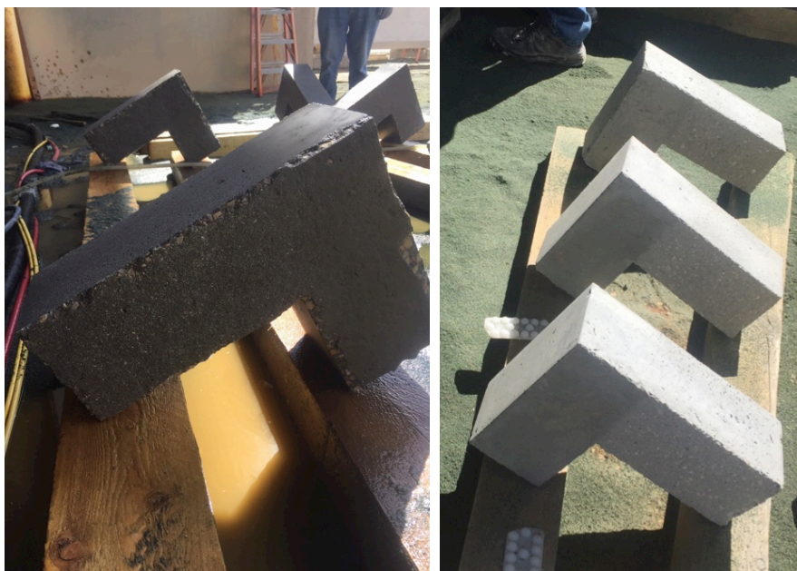
Figure 3.4 – Acid washed and media blasted specimens.
