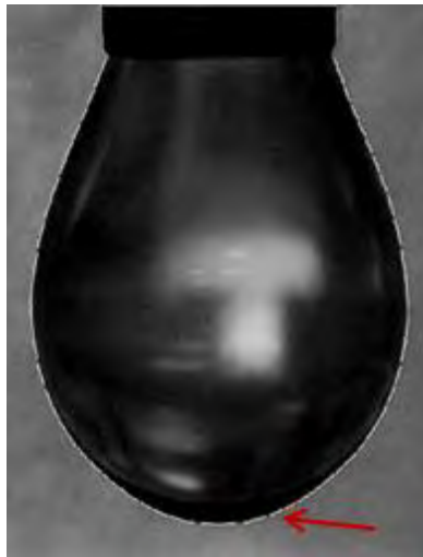
Figure 4.6: Formation of PFP lens at the apex of the water drop (red arrow).
