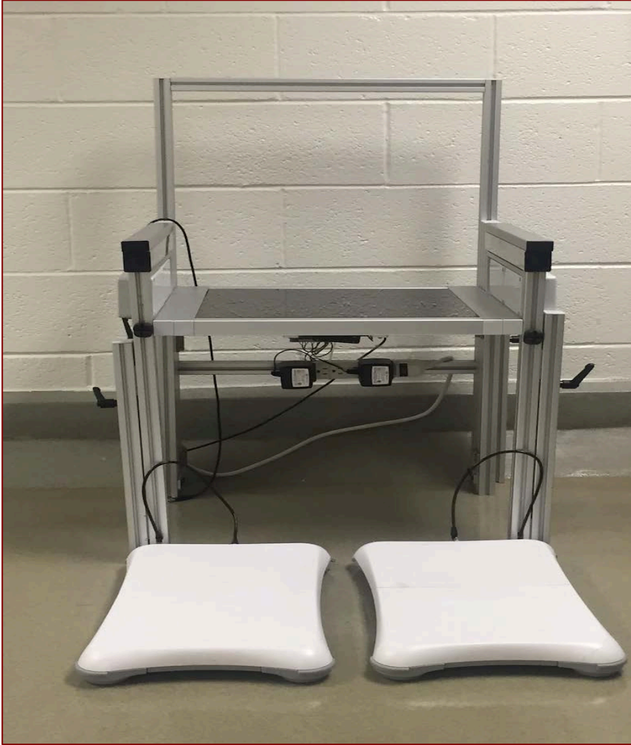
Figure 2.1. Instrumented Chair Designed for Sit-to-Stand Trials.
