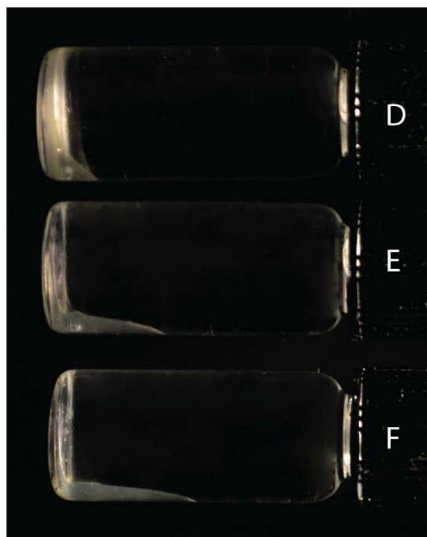
Figure 5.2: Photographs of coacervates to determine form and flow. NaCl concentration effects the transparency of coacervate: A) low salt (150 mM NaCl) resulted in cloudy coacervate, B) higher salt (1 M NaCl) results in a clear coacervate. C) Clear coacervates can be re-suspended into an emulsion of micro-coacervate droplets. D-F) The flow rate of coacervates is dependent on NaCl concentration: D) minimal flow in the gel-like coacervate with 150 mM NaCl, the flow rate increases with increasing NaCl concentration E) 500 mM NaCl and F) 1 M NaCl.
