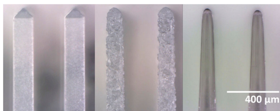
Fig. 6 (Left) Rough shaped optrodes after orthogonal dicing where the optrode dimensions are 150\mu\text{m} \times 1,600\mu\text{m} with a 45^\circ pyramidal tip. (Middle) Optrodes after 20 minutes of wet etching using a 5-minute pattern, repeated 4 times, of applying Armour Etch ® , rinsing with tap water, and drying with dry nitrogen/air. At this stage, the optrodes show substantial surface roughness from sodium and lime removal from the bulk of the soda lime glass by the fluoride ions of the Armour Etch ® paste. Optrodes have been reduced in size to 90\mu\text{m} \times 1,600\mu\text{m} . (Right) Polishing arrays greatly improves the surface roughness, while annealing helps mechanically strengthen optrodes. Final optrode dimensions are 100\mu\text{m} \times 1,100\mu\text{m} with a 37\mu\text{m} radius of curvature lens tip and a 2^\circ taper
