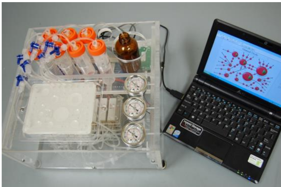
Figure 3.8: Completed PDMS extraction chip and control mechanism. This compact device uses electric vacuum and pressure pumps along with a bank of solenoid valves to control a PDMS microfluidic chip. A LabView control program allows easy adjustment of the protocol to handle a variety of sample inputs.
