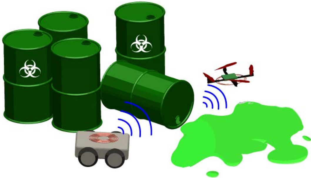
Figure 1.1: A potential use for a wirelessly powered MAV in a hazardous environment. A mobile ground robot might remain in close enough proximity to the MAV to allow it to return and charge [2].
