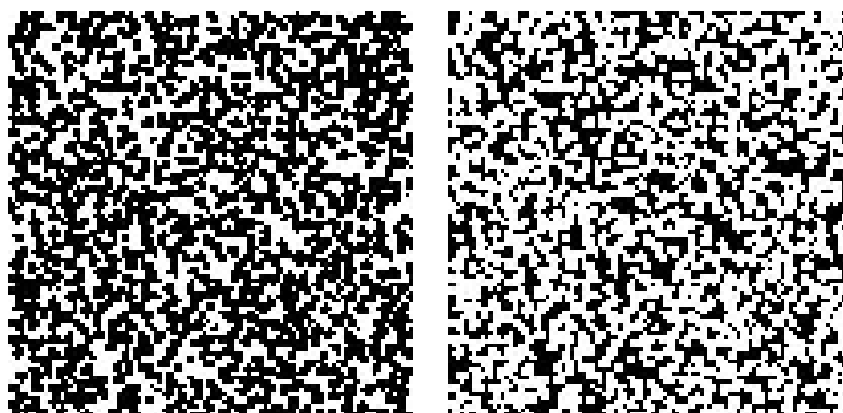
Figure 2.5 Illustration of a slice of the original raw image (left image) and a slice of the inverted image (right image). Black spots in the left image are water molecules and black spots in the right image are molecular pores.
