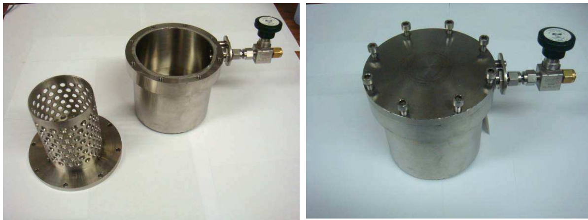
Figure 2.5.1: Shows the extraction vessel used in milling the ice core to release the trapped air bubbles.
