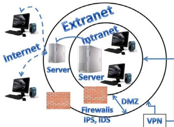
Figure 2 - Security Access Architecture Internet/Extranet/Intranet
