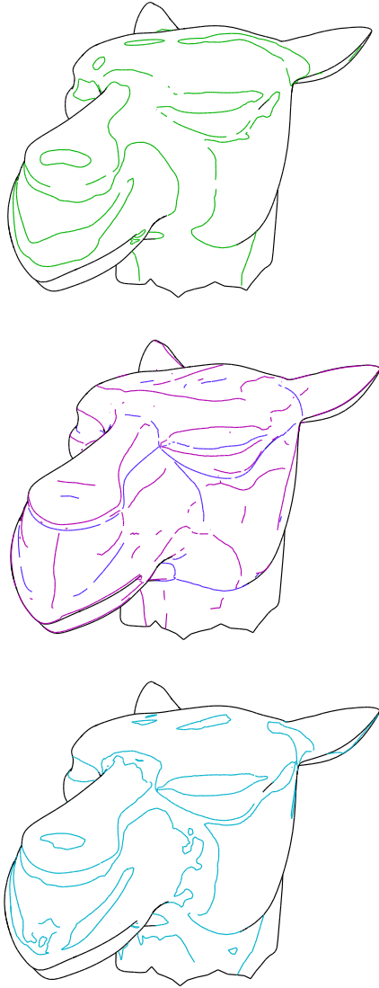
Figure 3: Camel head model with different line types, with filtering step disabled. From top to bottom : suggestive contours, ridges and valleys, demarcating curves. Occluding contours are in black.
