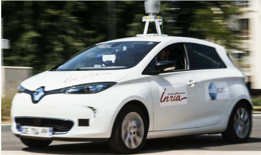
Fig. 4.6: Autonomous vehicle platform, Renault Zoe car, equipped with a Velodyne HDL-64 LiDAR
