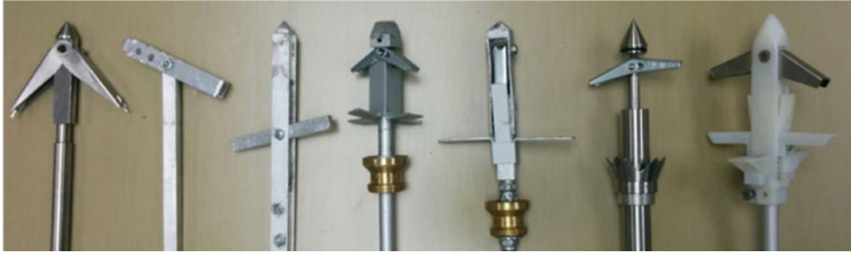
Figure 19. Harpoon tip and barbs design iteration.
