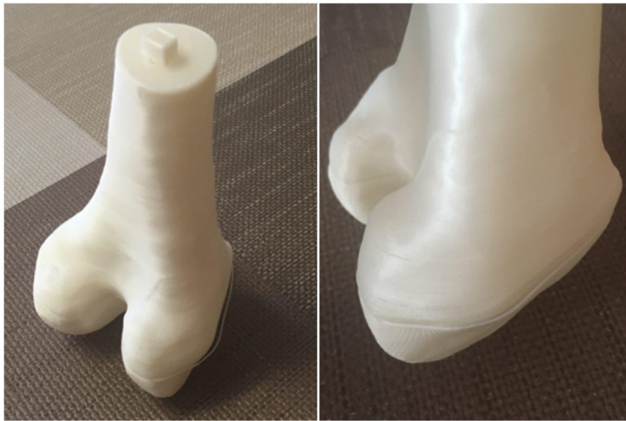
Figure 34. Bad layer adhesion issue.
