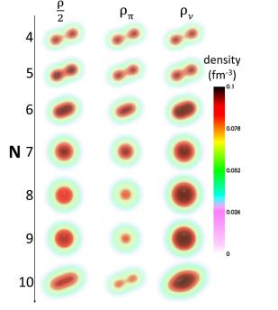
FIG. 7. (Color online) Total, proton, and neutron SCMF equilibrium intrinsic densities for beryllium isotopes, calculated using the RHB model with the functional DD-ME2.
