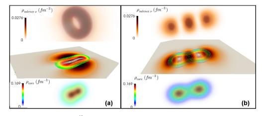
FIG. 9. (Color online) Intrinsic densities of <sup>10</sup>Be (a) at equilibrium deformation and (b) for an excited configuration. Bottom to top: 3D density of the  $\alpha + \alpha$  core, contour plots of the core density and the density of the valence neutrons in the (*Oxz*) plane, and 3D density of the valence neutrons.
