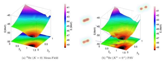
FIG. 5. (Color online) Self-consistent energy surfaces of <sup>8</sup>Be, calculated with DD-ME2 by (a) imposing constraints on both the axial quadrupole and octupole deformation parameters  $\beta_2$  and  $\beta_3$ , and (b) the corresponding positive parity-projected energy surfaces.
