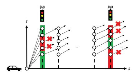
Figure 4.8: Optimization with respect to traffic light phases in the state graph. The yellow phases of the traffic lights are incorporated into the closest green phases. Through implicit discretization, the time of arrival at the traffic light can be computed. States that refer to a red phase are only feasible if the velocity component of the state is zero, i.e., the ego-vehicle stops. The ego-vehicle cannot continue while it is within a red phase.
