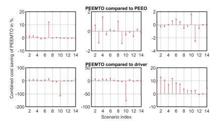
Figure 5.92: Combined cost saving of PEEMTO compared to PEEO and the ego-vehicle driver. Positive percental values mean PEEMTO leads to smaller costs. Negative percental values mean PEEMTO leads to higher costs. Rows top to bottom: PEEMTO compared to PEEO, PEEMTO compared to the ego-vehicle driver. Columns left to right: low traffic density, medium traffic density, high traffic density.
