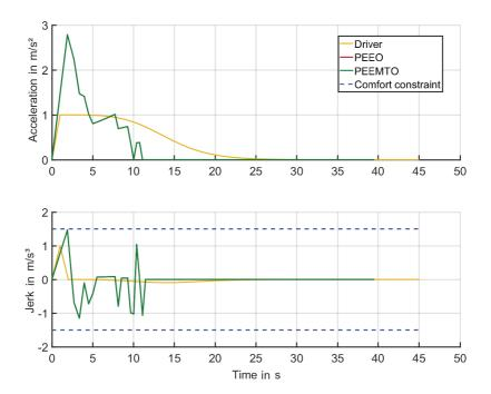
Figure 5.16: Optimization without explicit formulation of travel duration cost. Results of longitudinal acceleration and longitudinal jerk with respect to time for the egovehicle driver, PEEO, and PEEMTO. The results of PEEO and PEEMTO are identical and therefore overlap each other.
