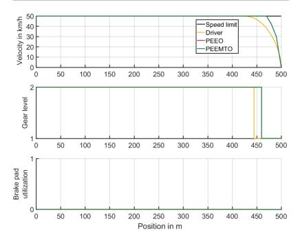
Figure 5.19: Deceleration without comfort constraints. Optimization results of velocity, gear level, and brake pad utilization with respect to position for the ego-vehicle driver, PEEO, and PEEMTO. The speed limit is set to  $50 \frac{\text{km}}{\text{h}}$ . The results of PEEO and PEEMTO are identical and therefore overlap each other.
