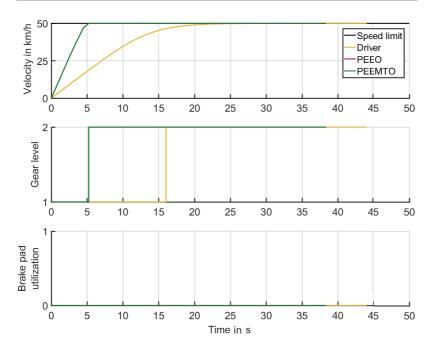
Figure 5.7: Acceleration without comfort constraints. Results of the ego-vehicle driver, PEEO, and PEEMTO with respect to time. The speed limit is set to 50  $\frac{kn}{h}$ . The results of PEEO and PEEMTO are identical and therefore overlap each other.
