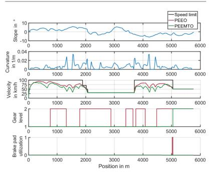
Figure 5.44: Scenario with fast front vehicle. Optimization results of velocity, gear level, and brake pad utilization with respect to position for PEEO, and PEEMTO. Similar results may overlap each other in the illustration.
