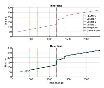
Figure 5.71: Optimization results of the time trajectory with respect to position. The yellow traffic light phases are incorporated into the green traffic light phases. Subtle velocity variations may not be conspicuous in the trajectory illustration. Similar or identical results may overlap each other.
