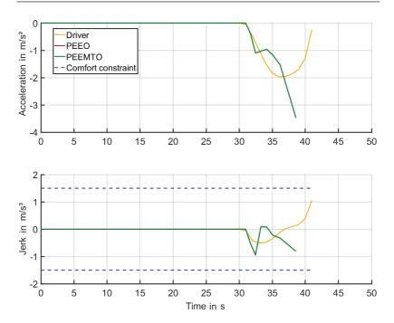
Figure 5.26: Deceleration with comfort constraints. Optimization results of longitudinal acceleration and longitudinal jerk with respect to time for the ego-vehicle driver, PEEO, and PEEMTO. The results of PEEO and PEEMTO are identical and therefore overlap each other.
