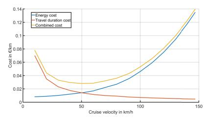
Figure 5.3: Cost at different cruise velocities. Energy consumption cost, travel duration cost, and combined cost with respect to different constant vehicle cruise velocities, at gear level two, on even, straight roads, over a distance of 1 km. The travel duration cost refers to a gross labor cost of  $0.7 \frac{e}{h}$ .
