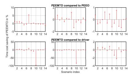
Figure 5.90: Travel duration cost saving of PEEMTO compared to PEEO and the ego-vehicle driver. Positive percental values mean PEEMTO leads to shorter travel durations. Negative percental values mean PEEMTO leads to longer travel durations. Rows top to bottom: PEEMTO compared to PEEO, PEEMTO compared to the ego-vehicle driver. Columns left to right: low traffic density, medium traffic density, high traffic density.
