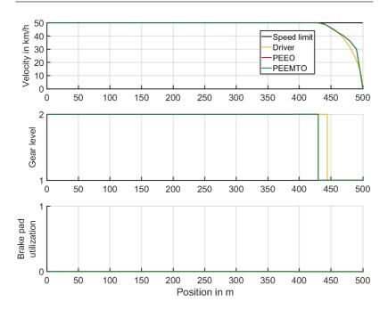
Figure 5.24: Deceleration with comfort constraints. Optimization results of velocity, gear level, and brake pad utilization with respect to position for the ego-vehicle driver, PEEO, and PEEMTO. The speed limit is set to  $50 \frac{\text{km}}{\text{h}}$ . The results of PEEO and PEEMTO are identical and therefore overlap each other.
