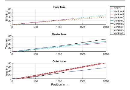
Figure 5.54: A8 highway scenario. Enlarged view of the trajectories of PEEO and the other vehicles in the inner, center, and outer lane.
