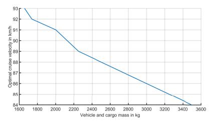
Figure 5.5: Optimal cruise velocity with respect to vehicle mass on even, straight roads. The travel duration cost refers to the minimum gross labor cost.
