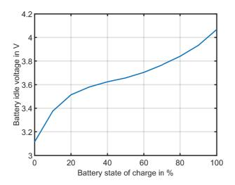
Figure 3.4: REM-2030 battery cell idle voltage depending on the battery state of charge.
