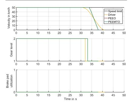
Figure 5.20: Deceleration without comfort constraints. Optimization results of velocity, gear level, and brake pad utilization with respect to time for the ego-vehicle driver, PEEO, and PEEMTO. The speed limit is set to 50  $\frac{\text{km}}{\text{h}}$ . The results of PEEO and PEEMTO are identical and therefore overlap each other.
