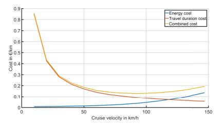
Figure 5.2: Cost at different cruise velocities. Energy consumption cost, travel duration cost, and combined cost with respect to different constant vehicle cruise velocities, at gear level two, on even, straight roads, over a distance of 1 km. The travel duration cost refers to the minimum gross labor cost of 8.5  $\frac{e}{b}$ .
