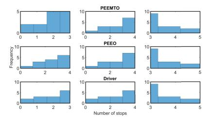
Figure 5.84: Distributions of complete stops. Rows top to bottom: PEEMTO, PEEO, egovehicle driver. Columns left to right: low traffic density, medium traffic density, high traffic density.
