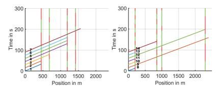
Figure 5.83: Left: Traffic light phases in the Ostring route. Right: Traffic light phases in the Adenauerring route. The start times are set within a range of 0 s to 90 s at 0 s, 15 s, 30 s, etc. The illustrated linear trajectories show how far the ego-vehicle can move for different start times until it is stopped by a red phase. Each start time represents one scenario. The scenario index is displayed next to the corresponding start time.
