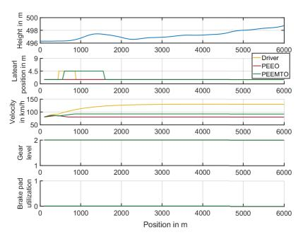
Figure 5.50: A8 highway scenario. Trajectories of the ego-vehicle driver, PEEO, and PEEMTO.
