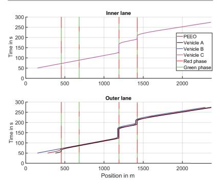
Figure 5.66: Optimization results of PEEO. Time trajectory with respect to position. The yellow traffic light phases are incorporated into the green traffic light phases. Subtle velocity variations may not be conspicuous in the trajectory illustration. Similar or identical results may overlap each other.
