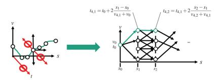
Figure 4.3: Implicit discretization of time. Explicit expansion of the time dimension is removed from the search space. Time progression is computed along possible velocity trajectories with respect to position.
