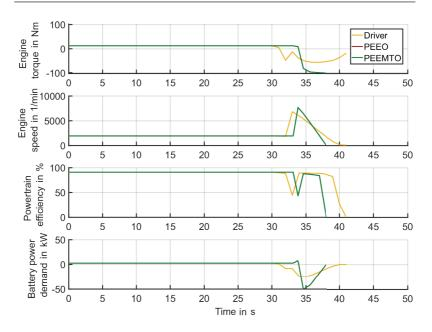
Figure 5.22: Deceleration without comfort constraints. Optimization results of engine torque, engine speed, powertrain efficiency, and battery power demand with respect to time for the ego-vehicle driver, PEEO, and PEEMTO. The results of PEEO and PEEMTO are identical and therefore overlap each other.
