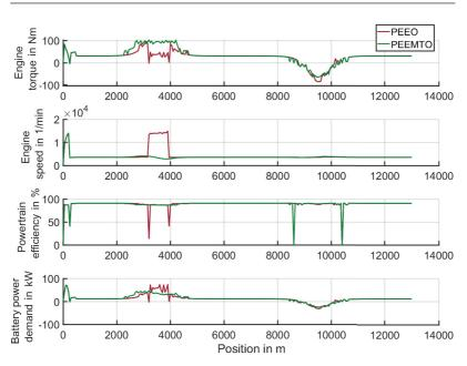
Figure 5.34: Optimization results of engine torque, engine speed, powertrain efficiency, and battery power demand with respect to time for PEEO and PEEMTO. Similar results may overlap each other in the illustration.
