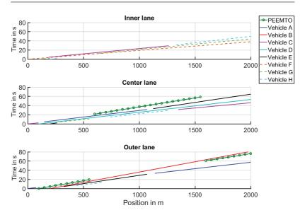
Figure 5.56: A8 highway scenario. Enlarged view of the trajectories of PEEMTO and the other vehicles in the inner, center, and outer lane.
