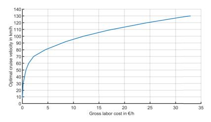
Figure 5.4: Optimal cruise velocities on even, straight roads, at gear level two, for different gross labor costs.
