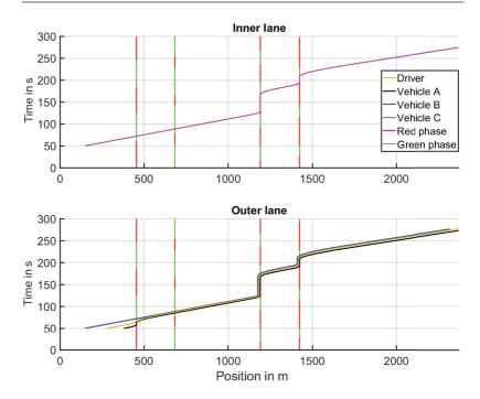
Figure 5.67: Optimization results of the ego-vehicle driver. Time trajectory with respect to position. The yellow traffic light phases are incorporated into the green traffic light phases. Subtle velocity variations may not be conspicuous in the trajectory illustration. Similar or identical results may overlap each other.
