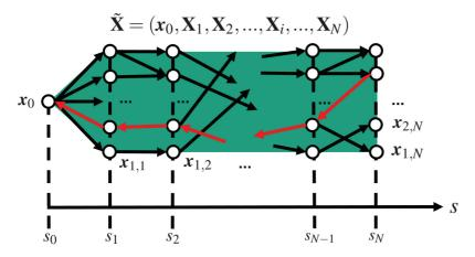
Figure 4.2: Structure of regular state graph used in PEEMTO. The green colored background of the state graph represents the abstract symbolic illustration of the state graph. States are represented by circles. Black arrows represent state transitions. Red arrows represent DP backtracing.
