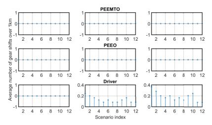
Figure 5.76: Average number of gear shifts over one kilometer. Rows top to bottom: PEEMTO compared to PEEO, PEEMTO compared to the ego-vehicle driver. Columns left to right: low traffic density, medium traffic density, high traffic density.
