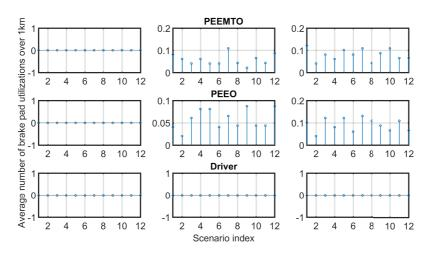
Figure 5.77: Average number of brake pad utilizations over one kilometer. Rows top to bottom: PEEMTO compared to PEEO, PEEMTO compared to the ego-vehicle driver. Columns left to right: low traffic density, medium traffic density, high traffic density.
