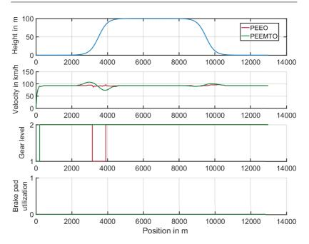
Figure 5.32: Height of road with respect to position. Optimization results of velocity, gear level, and brake pad utilization with respect to position for PEEO and PEEMTO. There is no speed limit and no road curvature. Similar results may overlap each other in the illustration.
