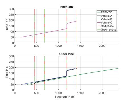
Figure 5.65: Optimization results of PEEMTO. Time trajectory with respect to position. The yellow traffic light phases are incorporated into the green traffic light phases. Subtle velocity variations may not be conspicuous in the trajectory illustration. Similar or identical results may overlap each other.
