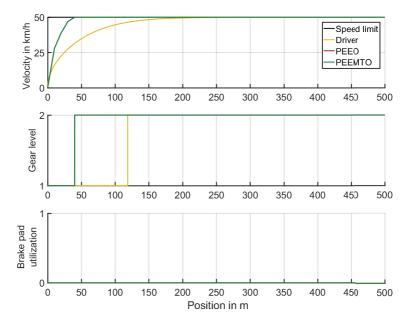
Figure 5.6: Acceleration without comfort constraints. Results of the ego-vehicle driver, PEEO, and PEEMTO with respect to position. The speed limit is set to 50  $\frac{km}{h}$ . Similar results may overlap each other in the illustration.
