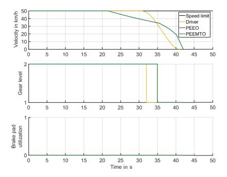
Figure 5.27: Deceleration without explicit formulation of minimum travel duration cost. Optimization results of velocity, gear level, and brake pad utilization with respect to time for the ego-vehicle driver, PEEO, and PEEMTO. The speed limit is set to  $50 \frac{\text{km}}{\text{h}}$ . The results of PEEO and PEEMTO are identical and therefore overlap each other.
