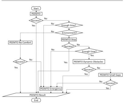
Figure 4.15: Flow diagram of PEEMTO dealing with cases, in which a solution cannot be successfully found. Depending on the reason of failure, the optimization is repeated with certain constraints adapted or removed. This can only happen if there is still enough computation time left. In the worst case scenario, emergency braking is suggested.
