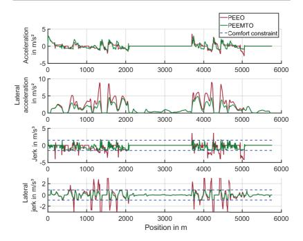
Figure 5.38: Short auxiliary horizon start length. Optimization results of longitudinal acceleration, lateral acceleration, longitudinal jerk, and lateral jerk with respect to position for PEEO and PEEMTO. Similar results may overlap each other in the illustration.
