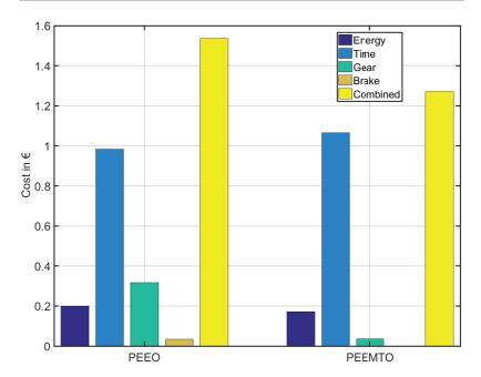
Figure 5.47: Scenario with fast front vehicle. Resulting costs of PEEO and PEEMTO at the end of the experiment.
