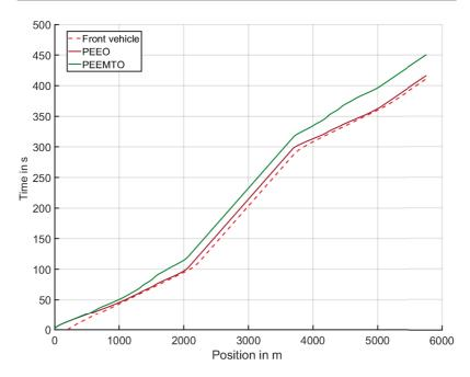
Figure 5.45: Scenario with fast front vehicle. Trajectories of position and time for the front vehicle, PEEO, and PEEMTO.
