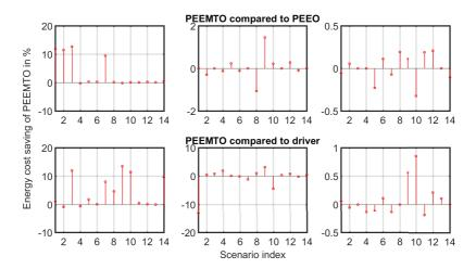
Figure 5.91: Energy consumption cost saving of PEEMTO compared to PEEO and the egovehicle driver. Positive percental values mean PEEMTO leads to smaller costs. Negative percental values mean PEEMTO leads to higher costs. Rows top to bottom: PEEMTO compared to PEEO, PEEMTO compared to the ego-vehicle driver. Columns left to right: low traffic density, medium traffic density, high traffic density.
