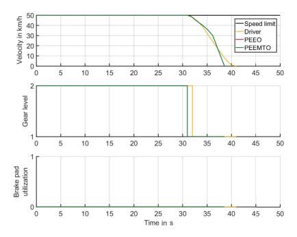
Figure 5.25: Deceleration with comfort constraints. Optimization results of velocity, gear level, and brake pad utilization with respect to time for the ego-vehicle driver, PEEO, and PEEMTO. The speed limit is set to  $50 \frac{\text{km}}{\text{h}}$ . The results of PEEO and PEEMTO are identical and therefore overlap each other.
