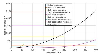
Figure 5.1: Resistance forces with respect to vehicle velocity.
