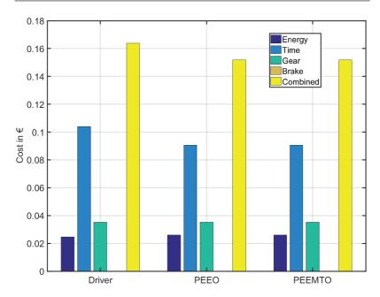
Figure 5.10: Acceleration without comfort constraints. Resulting costs of the different contenders at the end of the experiment without comfort consideration.
