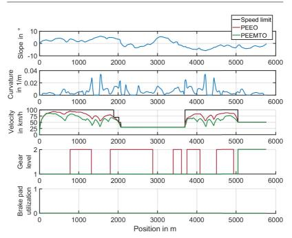
Figure 5.41: Scenario with long auxiliary horizon start length. Optimization results of velocity, gear level, and brake pad utilization with respect to position for PEEO and PEEMTO. Similar results may overlap each other in the illustration.
