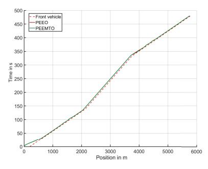
Figure 5.43: Scenario with slow front vehicle. Trajectories of position and time for the front vehicle, PEEO, and PEEMTO.
