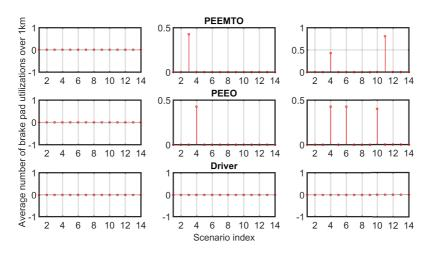
Figure 5.89: Brake pad utilizations. Rows top to bottom: PEEMTO compared to PEEO, PEEMTO compared to the ego-vehicle driver. Columns left to right: low traffic density, medium traffic density, high traffic density.
