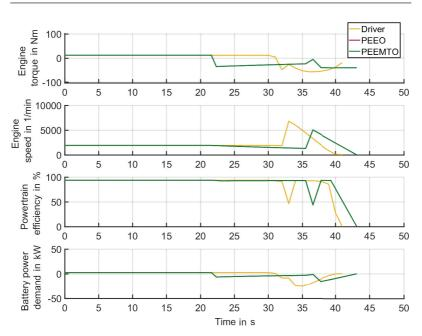
Figure 5.28: Deceleration without explicit formulation of minimum travel duration cost. Optimization results of engine torque, engine speed, powertrain efficiency, and battery power demand with respect to time for the ego-vehicle driver, PEEO and PEEMTO. The speed limit is set to 50  $\frac{\text{km}}{\text{h}}$ . The results of PEEO and PEEMTO are identical and therefore overlap each other.
