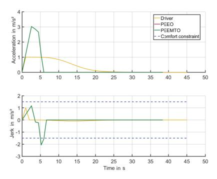
Figure 5.8: Acceleration without comfort constraints. Results of the ego-vehicle driver, PEEO, and PEEMTO. Comfort constraints refer to jerks of 1.5  $\frac{m}{s^3}$  and -1.5  $\frac{m}{s^3}$ . The results of PEEO and PEEMTO are identical and therefore overlap each other.
