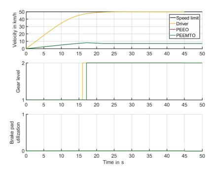
Figure 5.14: Optimization without any travel duration cost. Results of the ego-vehicle driver, PEEO, and PEEMTO. The speed limit is set to  $50 \frac{\text{km}}{\text{h}}$ . The results of PEEO and PEEMTO are identical and therefore overlap each other.
