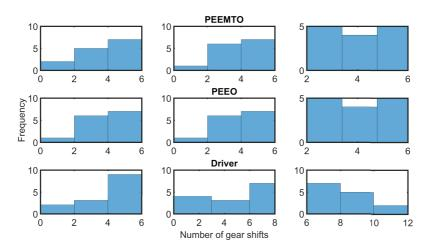
Figure 5.87: Distributions of gear shifts. Rows top to bottom: PEEMTO, PEEO, ego-vehicle driver. Columns left to right: low traffic density, medium traffic density, high traffic density.
