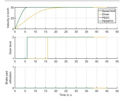
Figure 5.12: Acceleration with comfort constraints. Results of the ego-vehicle driver, PEEO and PEEMTO with respect to time. The speed limit is set to 50  $\frac{\text{km}}{\text{h}}$ . The results of PEEO and PEEMTO are identical and therefore overlap each other.
