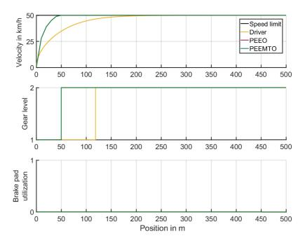
Figure 5.11: Acceleration with comfort constraints. Results of the ego-vehicle driver, PEEO and PEEMTO with respect to position. The speed limit is set to 50  $\frac{\text{km}}{\text{h}}$ . Similar results may overlap each other in the illustration.
