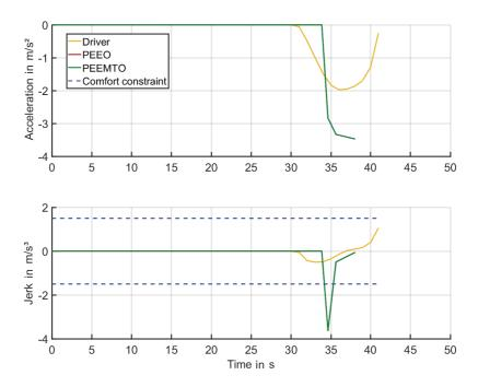
Figure 5.21: Deceleration without comfort constraints. Longitudinal acceleration and jerk with respect to time for the ego-vehicle driver, PEEO, and PEEMTO. The results of PEEO and PEEMTO are identical and therefore overlap each other.
