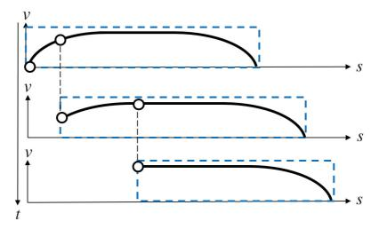
Figure 4.10: Illustration of trajectory optimization without terminal cost. The finite horizon is illustrated as a blue box with dashed edges. The computed velocity trajectory resides within the horizon. The horizon moves along with the ego-vehicle. Without a terminal cost, the velocity will usually drop to some extent at the end of the horizon because deceleration often leads to less energy consumption.
