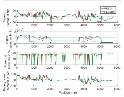
Figure 5.46: Scenario with fast front vehicle. Optimization results of engine torque, engine speed, powertrain efficiency, and battery power demand with respect to time for PEEO, and PEEMTO. Similar results may overlap each other in the illustration.
