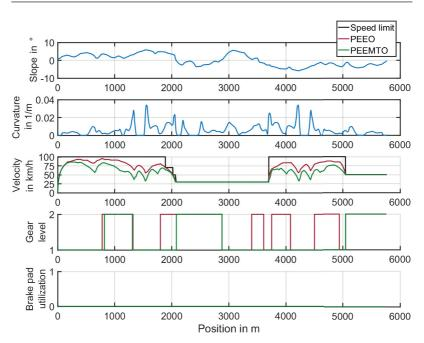
Figure 5.37: Scenario with short auxiliary horizon start length. Optimization results of velocity, gear level and brake pad utilization with respect to position for PEEO and PEEMTO. Similar results may overlap each other in the illustration.
