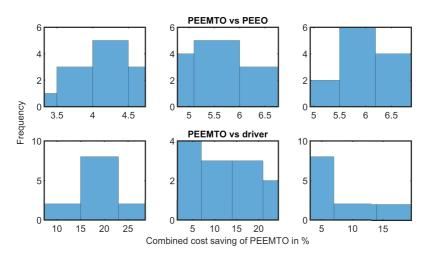
Figure 5.80: Combined cost of PEEMTO compared to PEEO and the ego-vehicle driver. Positive percental values mean PEEMTO leads to smaller costs. Negative percental values mean PEEMTO leads to higher costs. Rows top to bottom: PEEMTO compared to PEEO, PEEMTO compared to the ego-vehicle driver. Columns left to right: low traffic density, medium traffic density, high traffic density.
