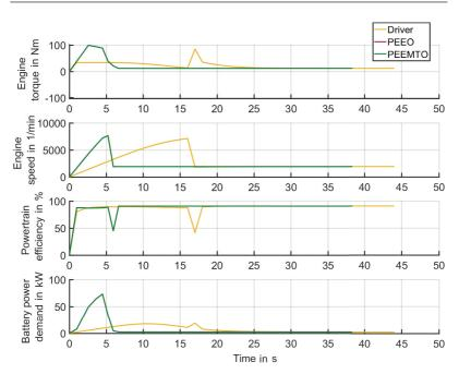
Figure 5.9: Acceleration without comfort constraints. Results of the ego-vehicle driver, PEEO, and PEEMTO. The results of PEEO and PEEMTO are identical and therefore overlap each other.
