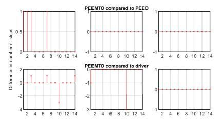
Figure 5.85: Reduction of stops. PEEMTO compared to PEEO and the ego-vehicle driver. A positive difference means PEEMTO leads to fewer stops. A negative difference means PEEMTO leads to more stops. Rows top to bottom: PEEMTO, PEEO, ego-vehicle driver. Columns left to right: low traffic density, medium traffic density, high traffic density.
