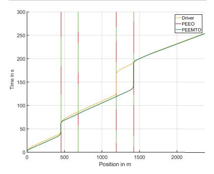
Figure 5.60: Optimization results of scenario in section 5.7.1. The illustration shows different time trajectories with respect to position. The yellow traffic light phases are incorporated into the green traffic light phases. Subtle velocity variations may not be conspicuous in the trajectory illustration. Similar results may overlap each other.
