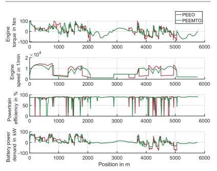
Figure 5.39: Scenario with short auxiliary horizon start length. Optimization results of engine torque, engine speed, powertrain efficiency, and battery power demand with respect to position for PEEO and PEEMTO. At gear level one, the engine speed is relatively high and resembles the velocity. At gear level two, the engine speed is significantly scaled down and the resemblance is less obvious. Similar results may overlap each other in the illustration.
