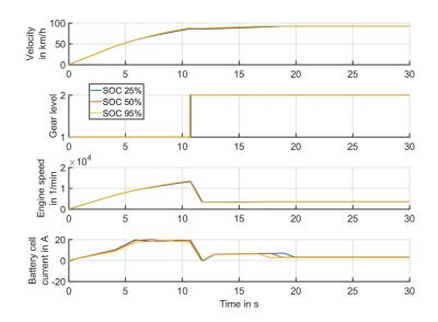
Figure 5.31: Acceleration of PEEMTO towards the optimal cruise velocity on even, straight roads at different states of charge (SOC). Similar results may overlap each other in the illustration.
