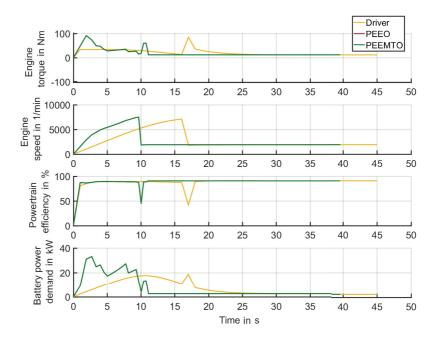
Figure 5.17: Optimization without explicit formulation of travel duration cost. Results of engine torque, engine speed, powertrain efficiency and battery power demand with respect to time for the ego-vehicle driver, PEEO, and PEEMTO. The results of PEEO and PEEMTO are identical and therefore overlap each other.
