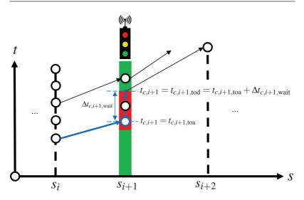
Figure 4.9: If the state transition leads into a red phase, the vehicle has to wait at the red traffic light until it turns green. In this case, a distinction between time of arrival and time of departure must be made.
