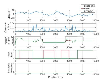
Figure 5.42: Scenario with slow front vehicle. Optimization results of velocity, gear level, and brake pad utilization with respect to position for PEEO and PEEMTO. Similar results may overlap each other in the illustration.
