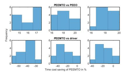
Figure 5.79: Travel duration cost of PEEMTO compared to PEEO and the ego-vehicle driver. Positive percental values mean PEEMTO leads to smaller costs. Negative percental values mean PEEMTO leads to higher costs. Rows top to bottom: PEEMTO compared to PEEO, PEEMTO compared to the ego-vehicle driver. Columns left to right: low traffic density, medium traffic density, high traffic density.
