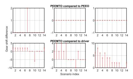
Figure 5.88: Gear shift savings of PEEMTO compared to PEEO and the ego-vehicle driver. Positive values mean PEEMTO has fewer gear shifts. Negative values mean PEEMTO has more gear shifts. Rows top to bottom: PEEMTO, PEEO, egovehicle driver. Columns left to right: low traffic density, medium traffic density, high traffic density.
