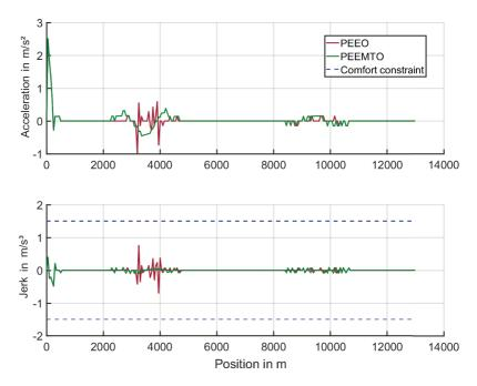
Figure 5.33: Optimization results of longitudinal acceleration and longitudinal jerk with respect to time for PEEO and PEEMTO. Similar results may overlap each other in the illustration.
