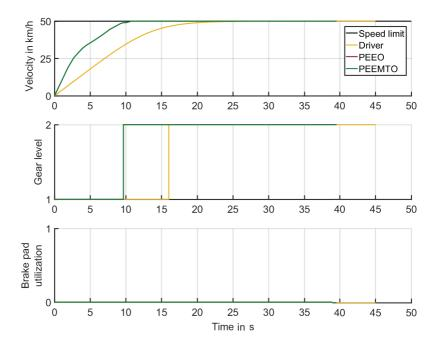
Figure 5.15: Optimization without explicit formulation of travel duration cost. Results of velocity, gear level, and brake pad utilization with respect to time for the egovehicle driver, PEEO, and PEEMTO. The speed limit is set to 50 km/h. The results of PEEO and PEEMTO are identical and therefore overlap each other.
