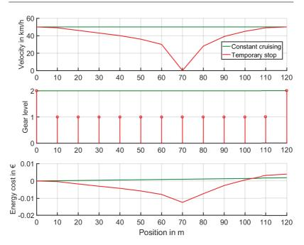
Figure 5.30: PEEMTO start and stop recuperation compared to constant cruising at optimal cruise velocity on an even and straight road. The speed limit set to  $50 \frac{\text{km}}{\text{h}}$ .
