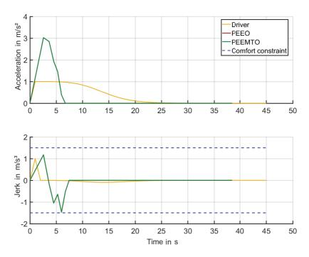
Figure 5.13: Acceleration with comfort constraints. Results of the ego-vehicle driver, PEEO and PEEMTO. Comfort constraints refer to jerks of  $1.5 \frac{m}{s^3}$  and  $-1.5 \frac{m}{s^3}$ . The results of PEEO and PEEMTO are identical and therefore overlap each other.
