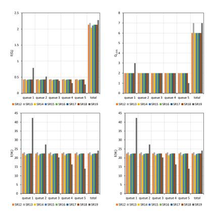
Figure 7.31: Expected value and 95%-quantile of the number of waiting customers and waiting time in the system per queue and total in case of no switching time from sink to queue with the same number and deterministic transitions for service rules with exhaustive service per queue
