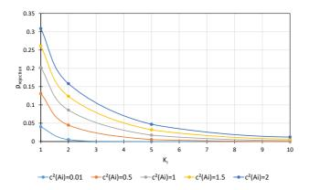
Figure 7.8: Impact of the queue capacity  $K_i$  with different interarrival time variabilities  $c^2(A_i)$  on the total rejection probability  $p_{reject}$
