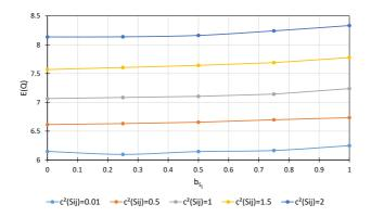
Figure 7.11: Impact of the distribution of the processing time over the queues measured by the gradient  $b_{S_i}$  with different processing time variabilities  $c^2(S_{ij})$  and processing time independent service rule (SR2) on the total queue length E(Q)
