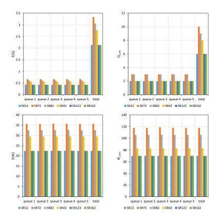
Figure 7.30: Expected value and 95%-quantile of the number of waiting customers and waiting time in the system per queue and total in case of no switching time from sink to queue with the same number and deterministic transitions for service rules with exhaustive or gated service per queue
