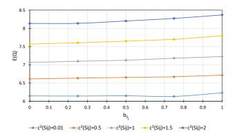
Figure 7.14: Impact of the distribution of the processing time over the sinks measured by the gradient  $b_{S_j}$  with different processing time variabilities  $c^2(S_{ij})$  on the total queue length E(Q)
