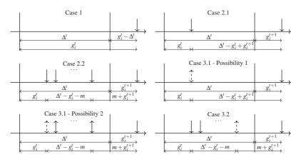
Figure 5.3: The different cases of transition of queue lengths and residual interarrival time for a time interval plotted in a time stream
