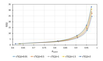
Figure 7.23: Impact of the utilization of the system  $\rho_{system}$  with different switching time variabilities  $c^2(C_{ii})$  on the total queue length E(Q)
