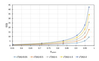
Figure 7.7: Impact of the utilization of the system  $\rho_{system}$  with different interarrival time variabilities  $c^2(A_i)$  on the total queue length E(Q)
