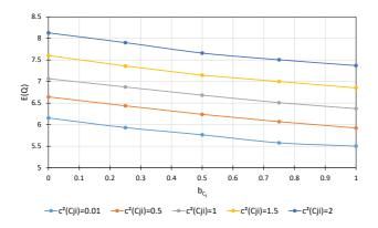
Figure 7.20: Impact of the distribution of the switching time over the sinks measured by the gradient  $b_{C_j}$  with different switching time variabilities  $c^2(C_{ji})$  and switching time dependent service rule (SR7) on the total queue length E(Q)
