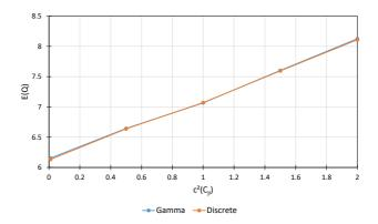
Figure 7.18: Impact of a higher switching time variability  $c^2(C_{ji})$  with different distribution types on the total queue length E(Q)
