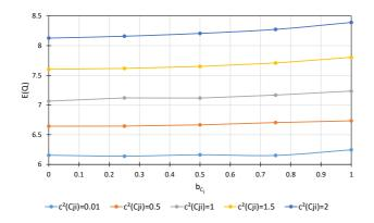
Figure 7.19: Impact of the distribution of the switching time over the sinks measured by the gradient  $b_{C_j}$  with different switching time variabilities  $c^2(C_{ji})$  and switching time independent service rule (SR2) on the total queue length E(Q)
