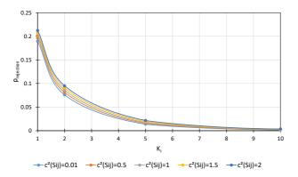
Figure 7.16: Impact of the queue capacity  $K_i$  with different processing time variabilities  $c^2(S_{ij})$  on the total rejection probability  $p_{reject}$
