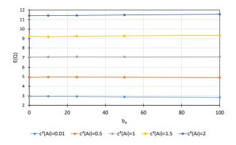
Figure 7.3: Impact of the distribution of arrivals over the queues measured by the gradient  $b_A$  with different interarrival time variabilities  $c^2(A_i)$  on the total queue length E(Q)
