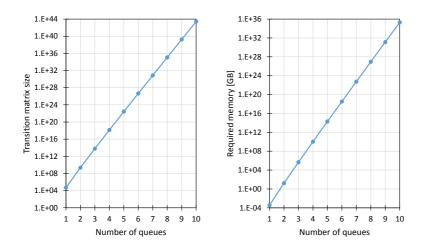
Figure 6.1: Development of the transition matrix size and the required memory for the transition matrix with an increasing number of queues
