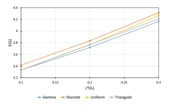
Figure 7.1: Impact of the interarrival time variability  $c^2(A_i)$  with different distribution types on the total queue length E(Q)
