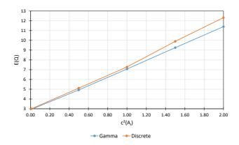
Figure 7.2: Impact of a higher interarrival time variability  $c^2(A_i)$  with different distribution types on the total queue length E(Q)
