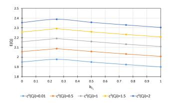
Figure 7.21: Impact of the distribution of the switching time over the sinks measured by the gradient  $b_{C_j}$  with different switching time variabilities  $c^2(S_{ji})$  and switching time dependent service rule (SR8) on the total queue length E(Q)
