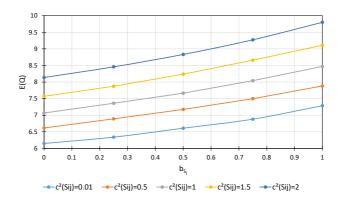
Figure 7.13: Impact of the distribution of the processing time over the queues measured by the gradient  $b_{S_i}$  with different processing time variabilities  $c^2(S_{ij})$  and processing time dependent service rule (SR8) on the total queue length E(Q)
