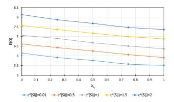
Figure 7.12: Impact of the distribution of the processing time over the queues measured by the gradient  $b_{S_i}$  with different processing time variabilities  $c^2(S_{ij})$  and processing time dependent service rule (SR7) on the total queue length E(Q)
