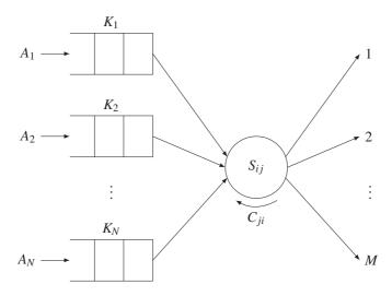
Figure 5.1: Multi-queue system with multiple departure streams (MQSMDS)
