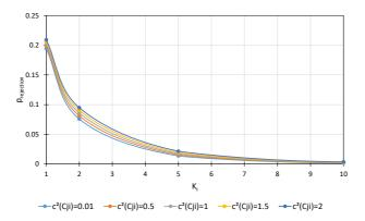
Figure 7.24: Impact of the queue capacity  $K_i$  with different switching time variabilities  $c^2(C_{ji})$  on the total rejection probability  $p_{reject}$
