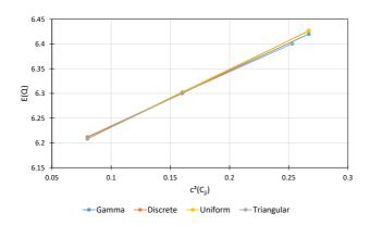
Figure 7.17: Impact of the switching time variability  $c^2(C_{ji})$  with different distribution types on the total queue length E(Q)
