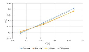
Figure 7.9: Impact of the processing time variability  $c^2(S_{ij})$  with different distribution types on the total queue length E(Q)
