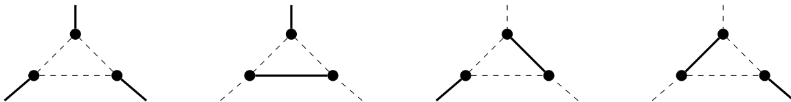
Figure 4: The different matchings for a triangle, where thick lines denote edges in the matching and dashed lines denote edges not in the matching.
