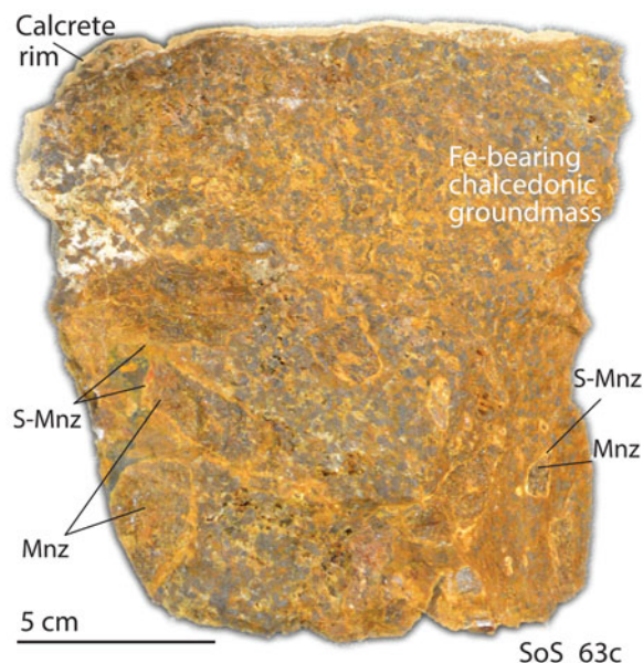
Fig. 2. Example of monazite-(Ce)-bearing (Mnz) silicified carbonatite from Eureka. Note the \sim 500 \mu\text{m} S-bearing monazite-(Ce) rims (S-Mnz) around the monazite-(Ce) grains.
