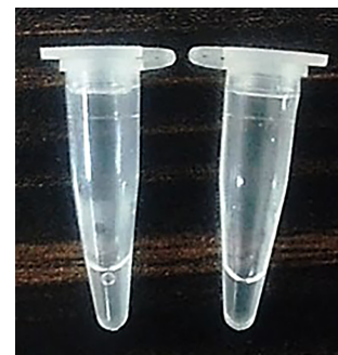
Figure 1. Positive (left) and negative (right) reactions of LAMP assay based on the presence of turbidity
