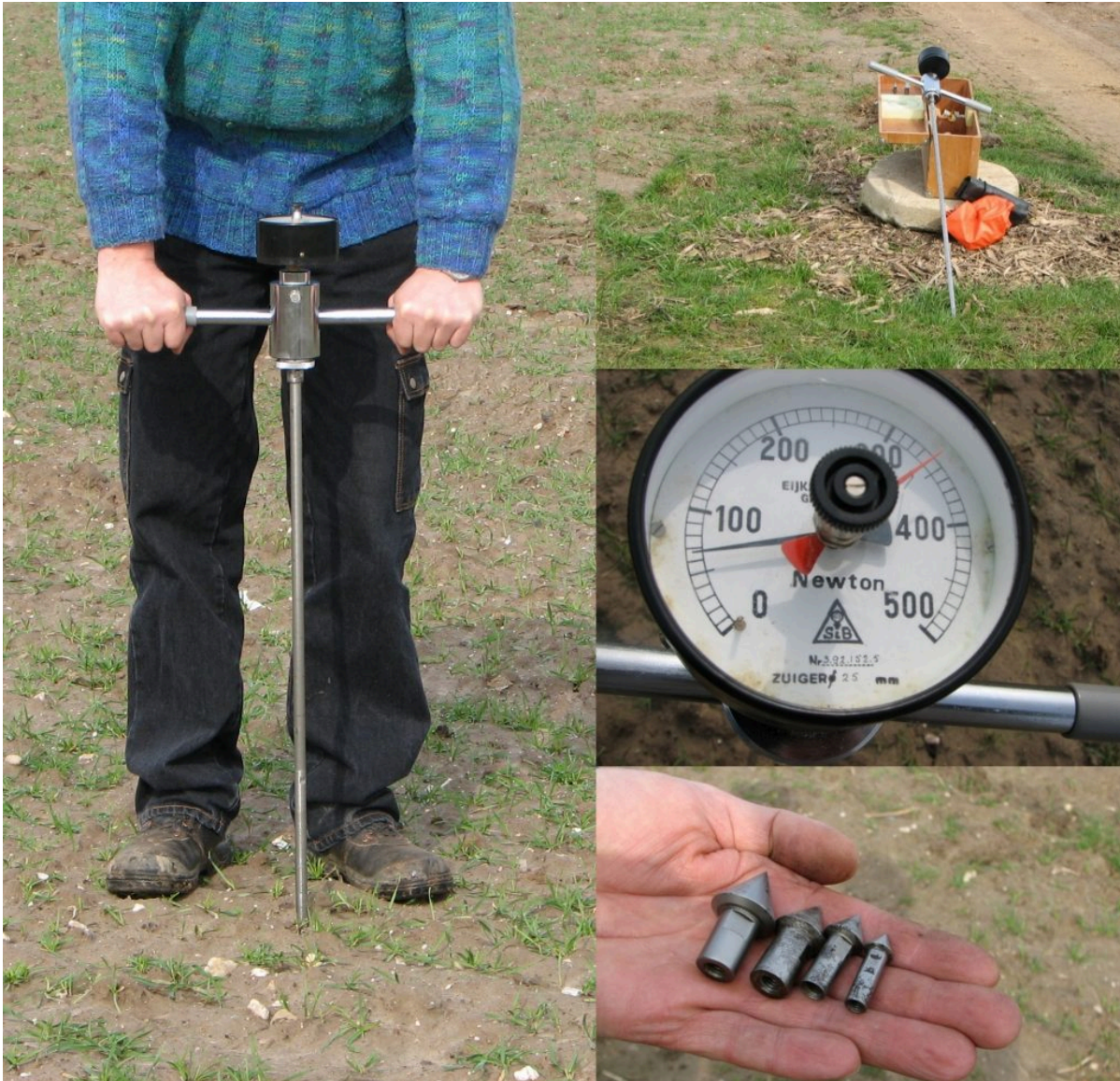
A handheld penetrometer being used in the field (left), associated equipment (top right), power meter (center right), and cones (bottom right). Photograph courtesy of HPsy.
