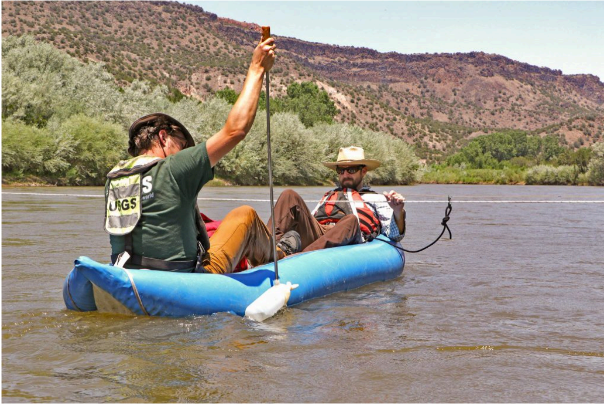
USGS scientists sampling for suspended-sediment concentration on the Rio Grande River. Photograph courtesy of the USGS.
