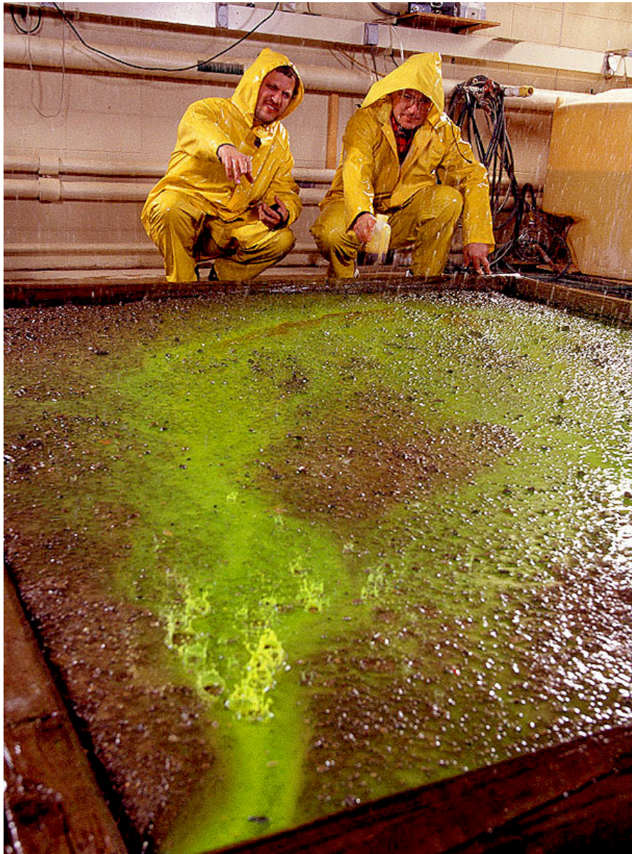
Two ARS researchers watch a rainfall simulation being used to improve the WEPP model used to predict erosion. Photograph by Scott Bauer, courtesy of the USDA ARS.
