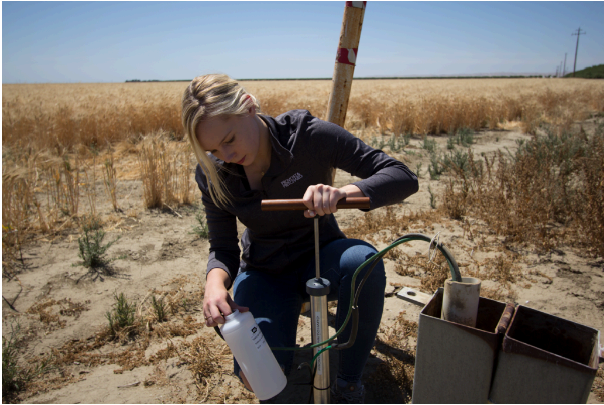
Collection of soil pore water from a pressure/vacuum sampler on the corner of a wheat field near Huron, California. Photograph by Philip Melcher, Provost & Pritchard Consulting Group.
