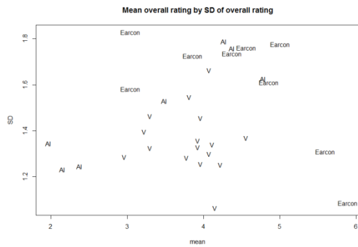
Figure 1: Mean overall rating against standard deviation of overall rating for each of the 32 stimuli (presented as warning “type”; V = verbal, Earcon, or AI = Auditory Icon). Based on this metric, the two highest performing (with the most agreement) stimuli are the low siren and high-pitched faster beeps earcon. Contrary to the authors’ hypothesis, the majority of auditory icons (featuring various actual train sounds) were either consistently rated as not appropriate (mean < 2, low SD), or inconsistently rated as averagely appropriate (mean between 3-5, high SD). An interesting pattern emerged from the ratings for verbal stimuli, as the majority (all but one) is clustered in the center of the plot. Comparing overall ratings by type (figure 2) shows that due to the high variance within type groups, no statistically significant difference in mean ratings can be found. A repeated measures analysis of variance was conducted on the verbal warnings to investigate the effect of word, gender, and
