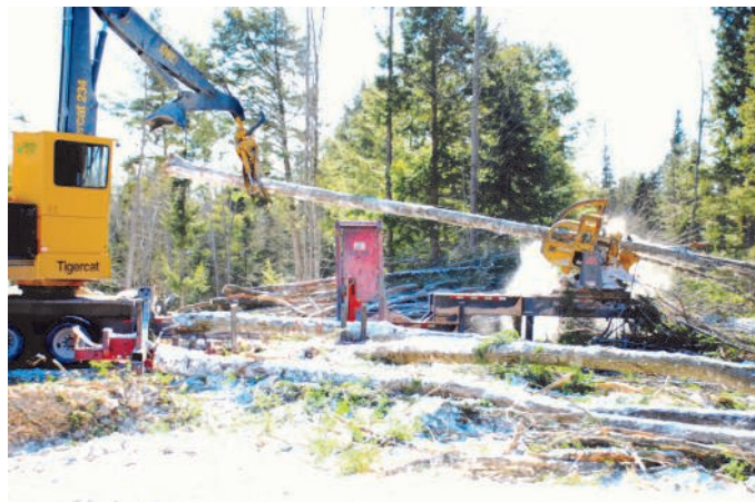
A crane pulls a tree through a delimeter at a Maine Custom Woodlands harvest site in New Gloucester. (Photo: Joe Rankin)
