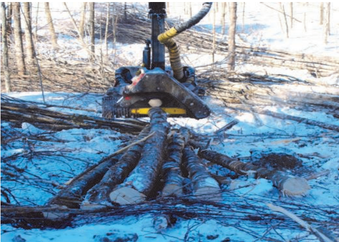
Dana Poulin runs wood through his dangle head cut to length system (Photo: Joe Rankin)
