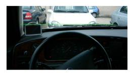
For safety reasons, the display should always be fixed to the car by means of a holder. Recommended is to place the display at dashboard level (see picture), to ensure that the display is not blocking the view of the driver.
