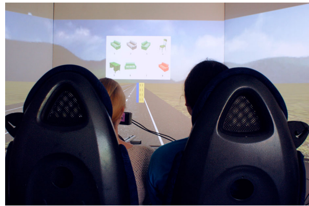
Figure 2. The driving simulator used for this experiment. Speaker-passengers described a target image from the image array displayed above the road. Listener-drivers had to follow the yellow bar back and forth across the road while identifying the intended referent by number.
